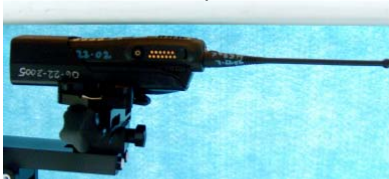
Figure 1: Highest S.A.R. Test Position (Face) Front of radio separated 2.5cm
