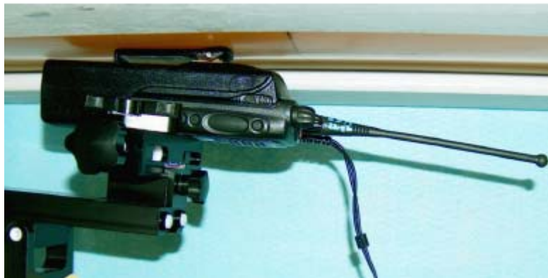
Figure 2: Highest S.A.R. Test Position (Body) Unit back against phantom Audio accessory model PMLN4418B attached.
