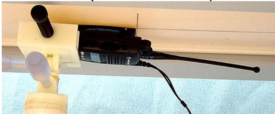
Figure 3: Assessment at the Abdomen; DUT w/ HLN9714A belt clip and attached audio accessory model PMLN4418A
