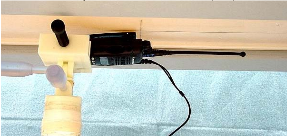
Figure 3. Highest S.A.R. configuration Run # Ab_R1_020308-05 S.A.R. performance assessment at abdomen (2.5cm)
