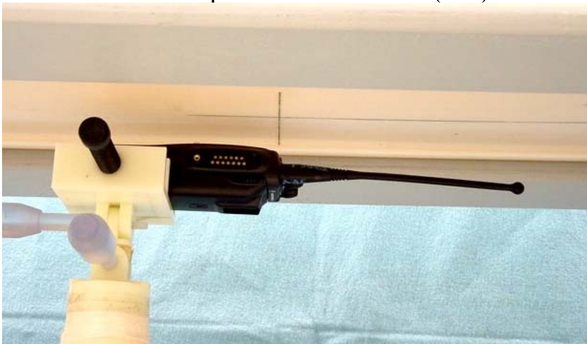
Figure 4. Highest S.A.R. configuration Run # Face_R1_020311-09 S.A.R. performance assessment at face (2.5cm)
