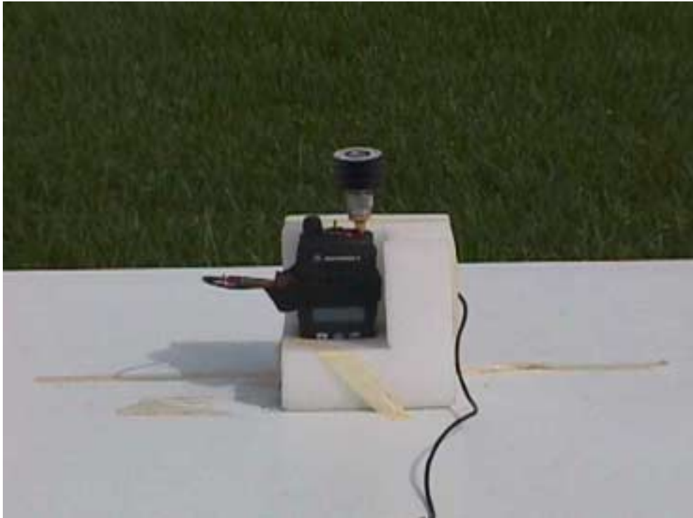
Figure 8 – OATS Device Under Test with Non-Radiating Load
