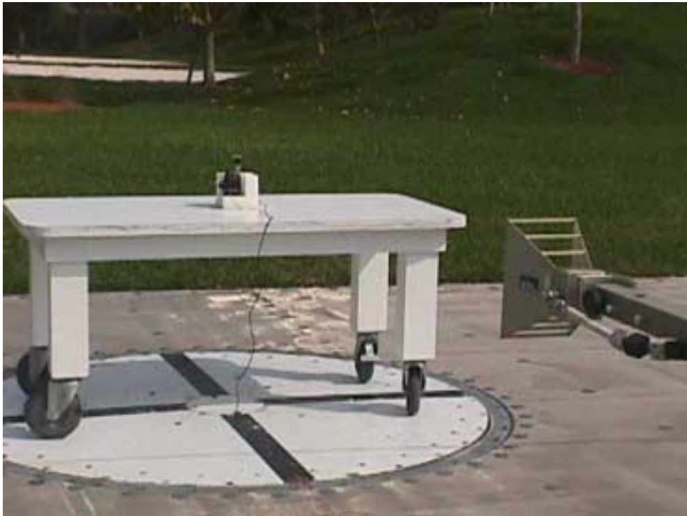
Figure 7 – OATS Radiated Spurious Emissions Test Setup
