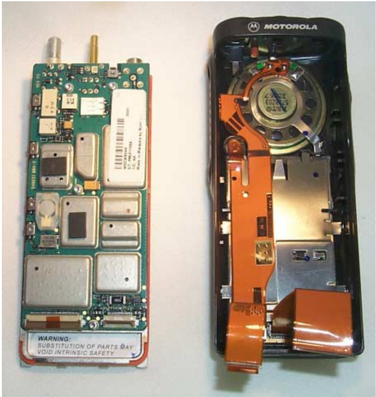
REAR VIEW WITH CIRCUIT BOARD REMOVED FROM HOUSING (MATING SURFACES OF BOARD AND HOUSING ARE SHOWN)
