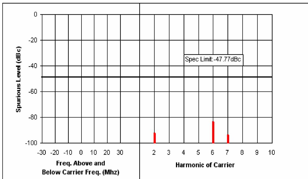
The conducted spurious level is plotted in dBc on the vertical axis.
