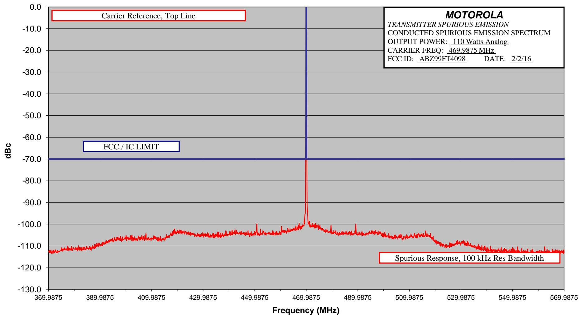
**Report on Test Measurements***Radiated Spurious Emissions, Harmonics*Specification Requirement 47 CFR §90.210(b) and IC RSS-119 section 5.8.1 - Emission Limits – “B-Mask”:
