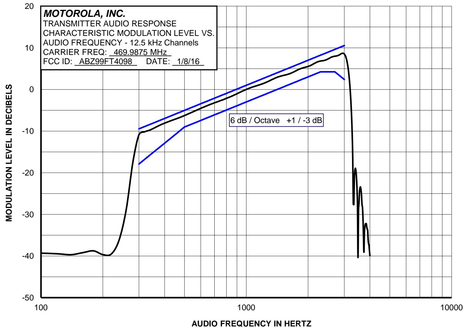
**Report on Test Measurements***Modulation Limiting*Specification Requirement per TIA 603:
