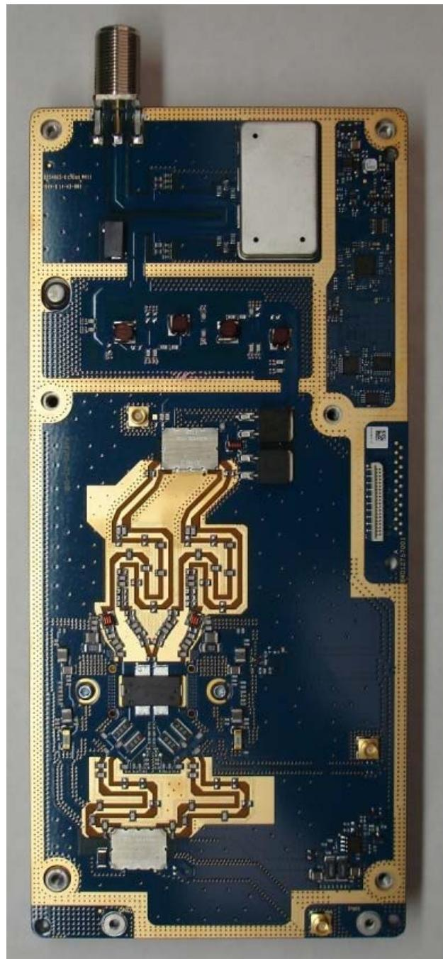
**Exhibit 9F – Internal Front View – Power Amplifier Module – Bottom View, Heat Sink Removed**
