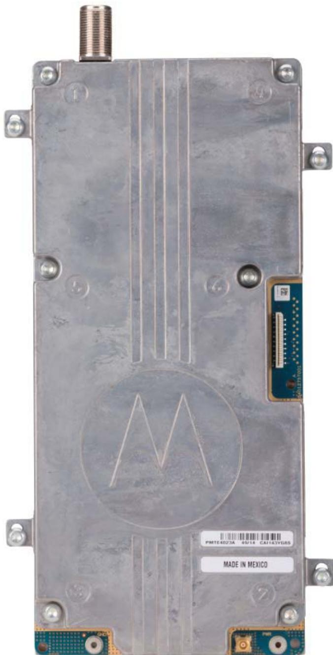
**Exhibit 9E – Internal Front View – Power Amplifier Module – Top View, Cover Removed**
