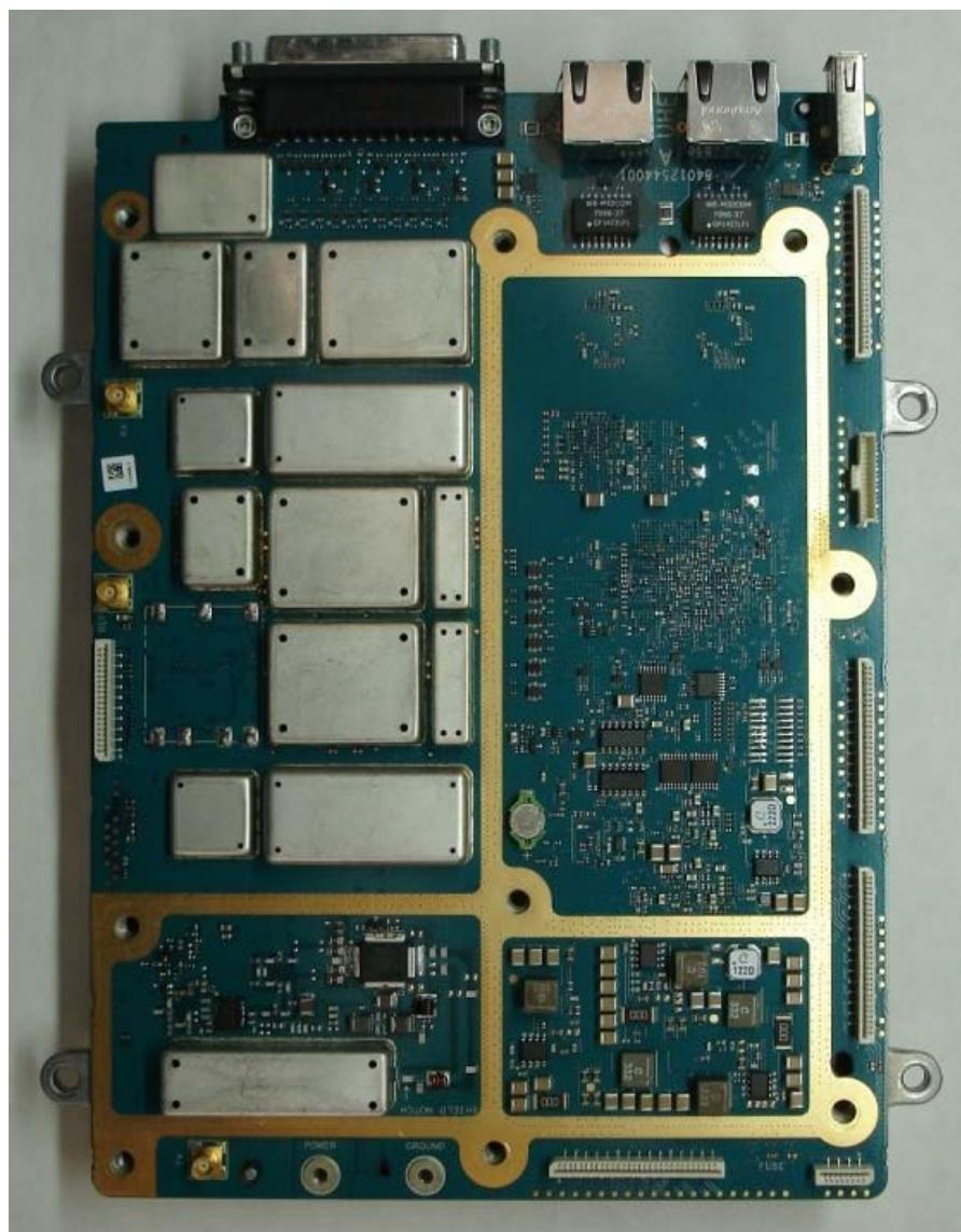
**Exhibit 9C – Internal Front View – Modem Module Bottom View – Heat Sink Removed**
