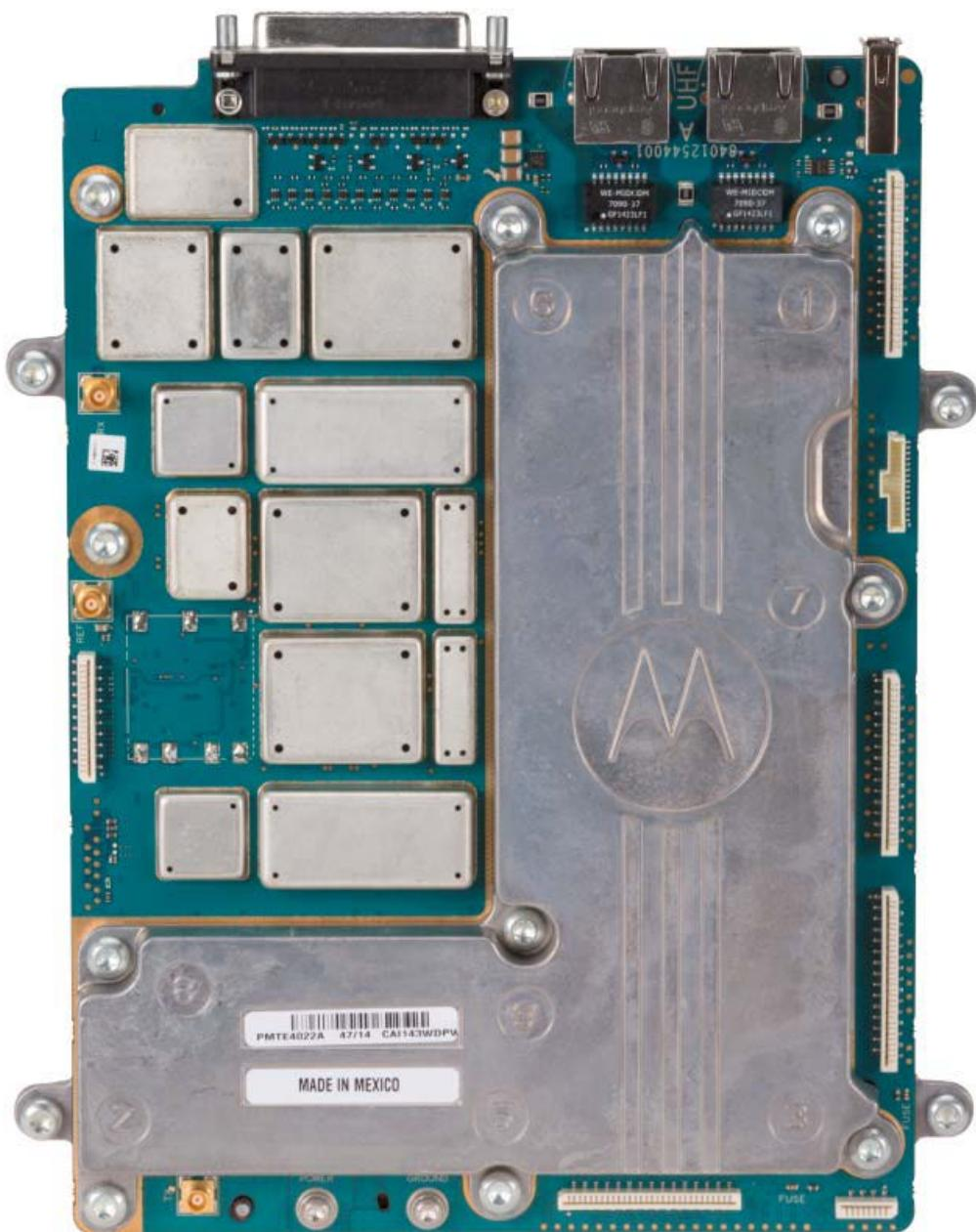
**Exhibit 9B – Internal Front View – Modem Module Top View – Cover Removed**
