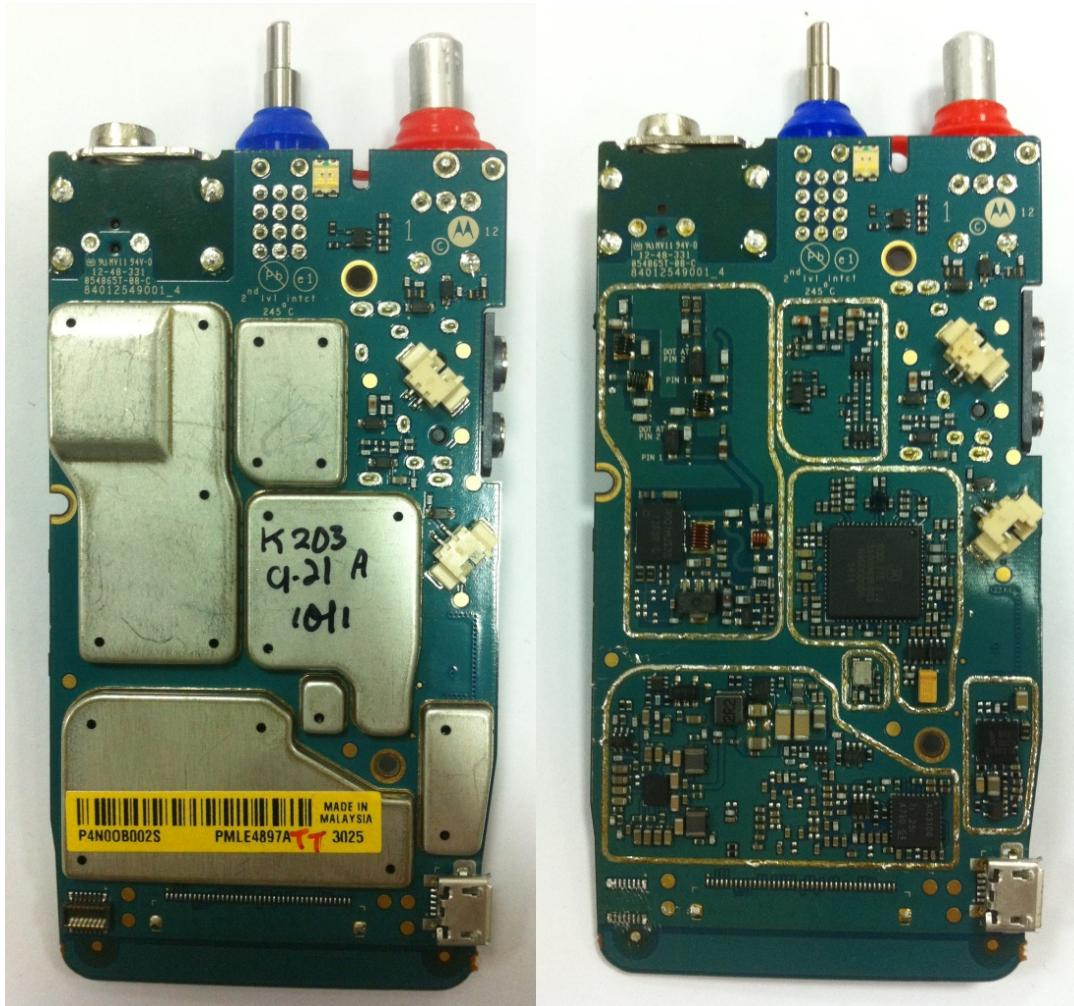
RF board with and without Shields (Top)
