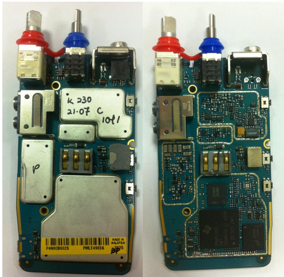
RF board with and without Shields (Bottom)
