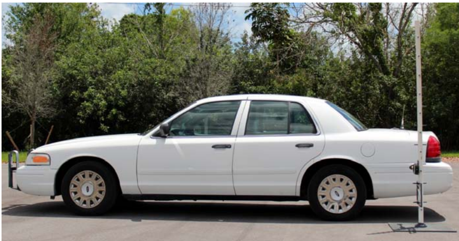
Test measurement setup for Bystander 90 degree (side) trunk mount antenna
