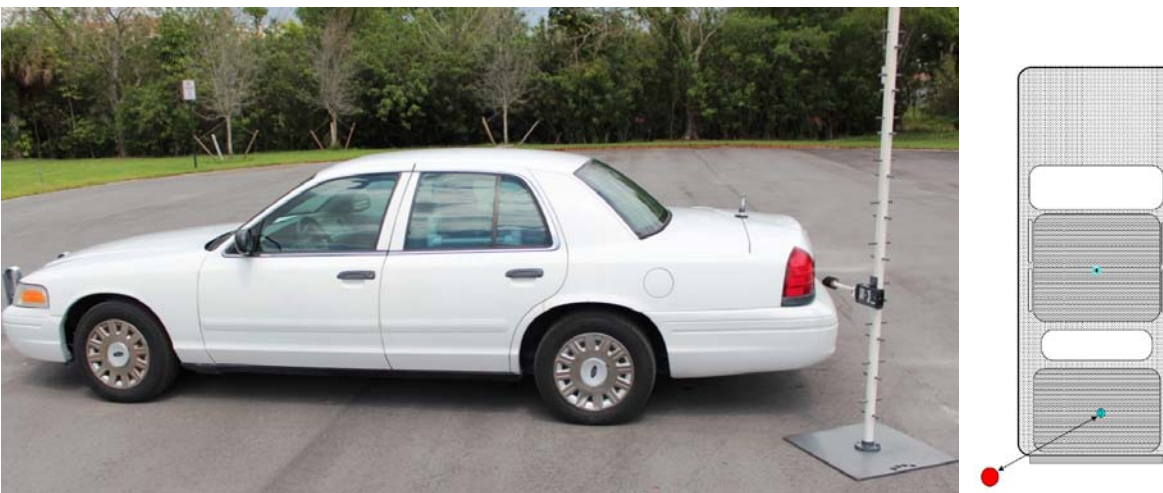
Test measurement setup for Bystander 45 degree (diagonal) trunk mount antenna
