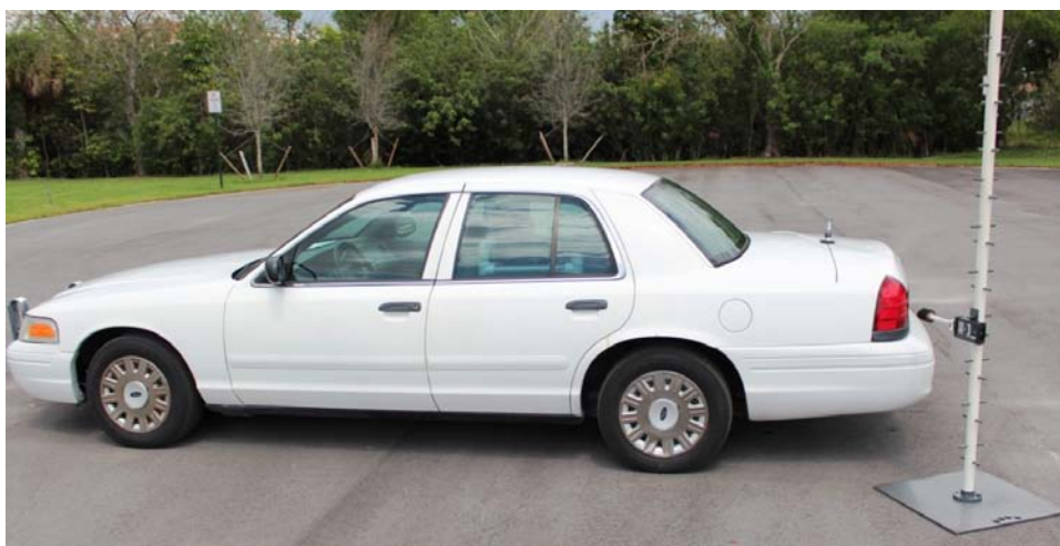
Test measurement setup for Bystander 45 degree (diagonal) trunk mount antenna
