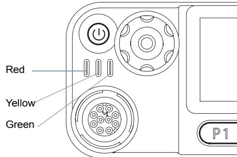
**Blinking red** – Radio is transmitting at low battery condition, receiving an emergency transmission or has failed the self-test upon powering up.
