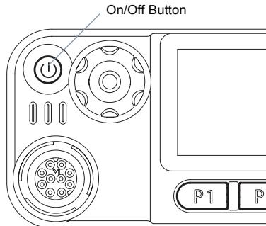
To turn off the radio, press and hold the On/Off Button until you see **Powering Down** on the radio's display.
