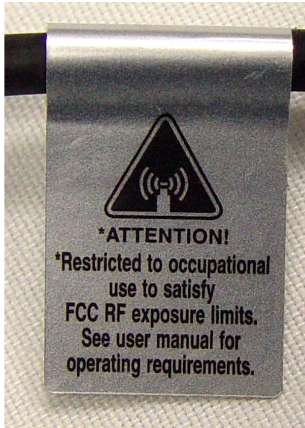
RF EXPOSURE LABEL (CLOSE-UP VIEW)
