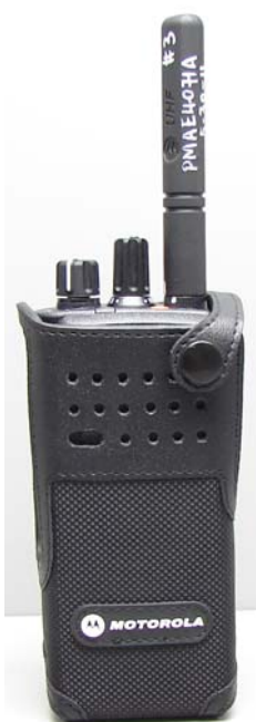
DUT Front View Nylon case PMLN5845A w/ fixed belt loop
