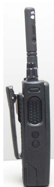
DUT Side View Belt clip PMLN7008A 2.5 inch
