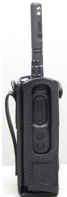
DUT Side View Nylon case PMLN5845A w/ fixed belt loop
