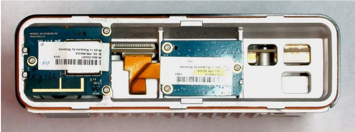
FRONT VIEW WITH BLUETOOTH/GPS BOARD INSTALLED ON THE LEFT AND GENERIC OPTION BOARD INSTALLED ON THE RIGHT
