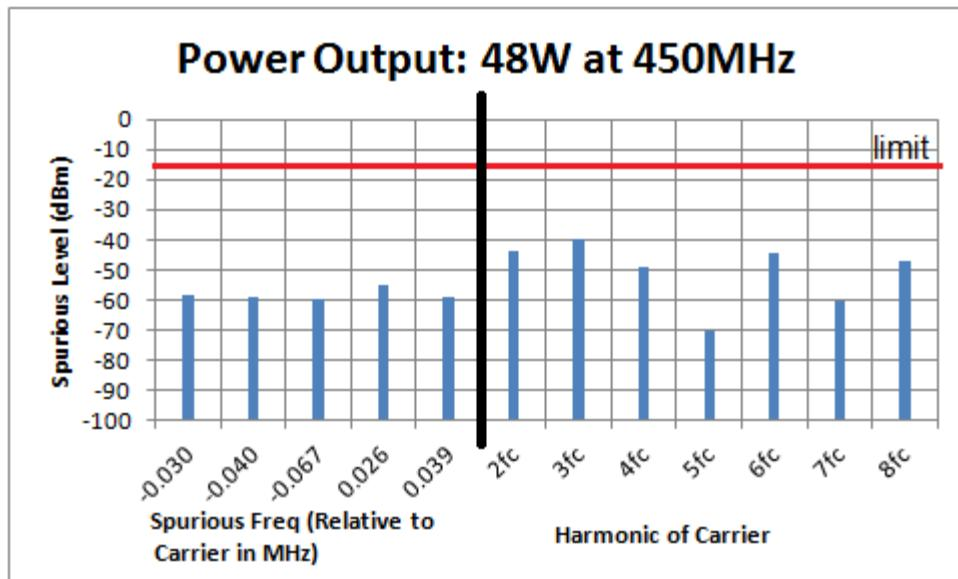
The conducted spurious level is plotted in dBm on the vertical axis.
