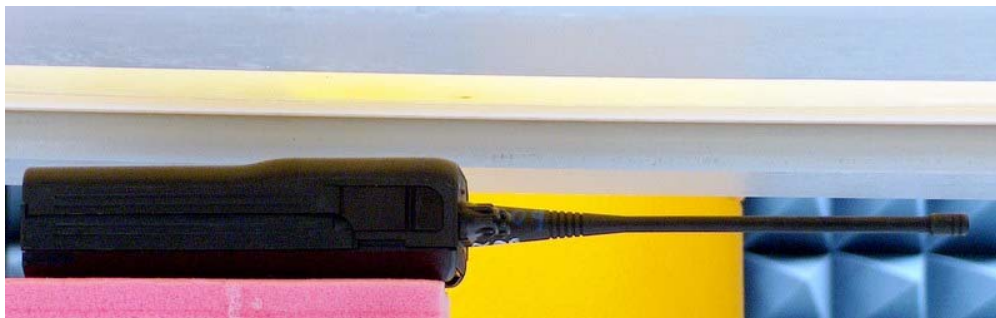
Figure 2: Highest SAR Test Position (Face) Antenna model NAE6483AR DUT front side separated 2.5cm from the phantom; no accessory attached.
