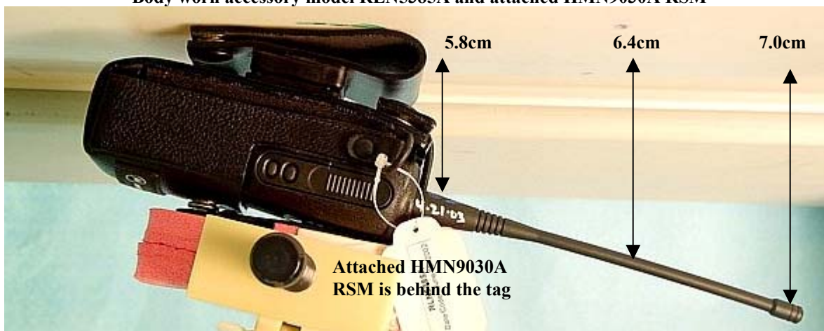
Figure 5: Assessment @ the Abdomen; DUT w/ Body worn accessory model RLN5385A and attached HMN9030A RSM
