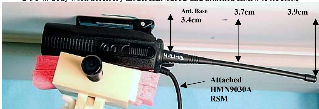
Figure 3. Assessment @ the Abdomen; DUT w/ body worn accessory model HLN8255B and attached HMN9030A RSM
