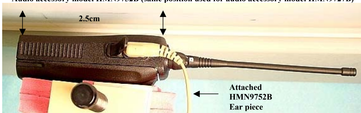
Figure 7: Assessment @ the Face; DUT front w/ 2.5cm separation Audio accessory model HMN9752B (same position used for audio accessory model HMN9727B)
