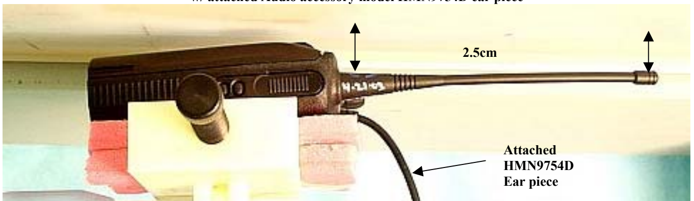
Figure 9: Assessment @ the Abdomen; DUT w/ antenna 2.5cm separation w/ attached Audio accessory model HMN9754D ear piece
