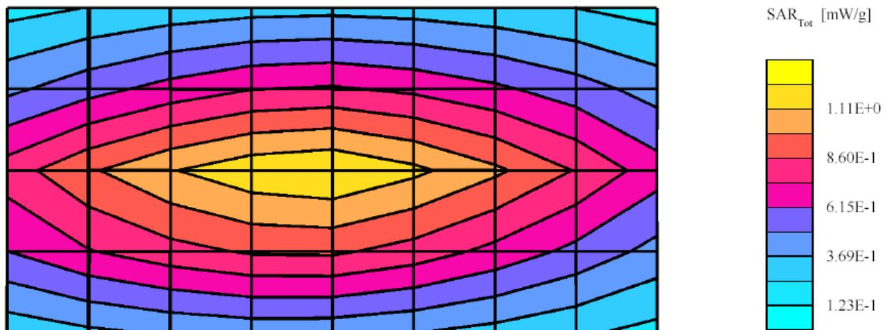
**SPEAG 450 MHz Dipole D450V2; SN-1002; Test Date: 9/02/03**
