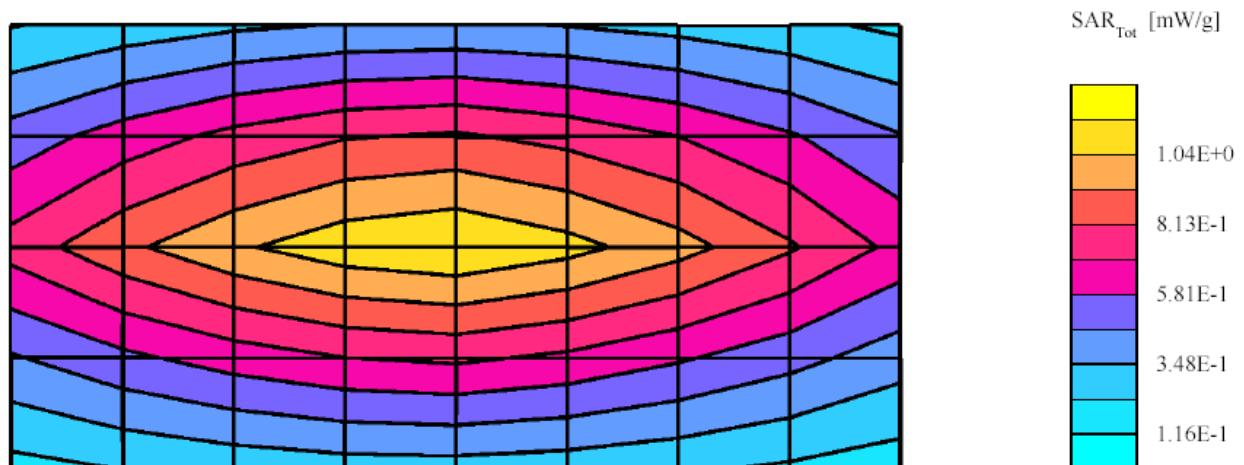
**SPEAG 450 MHz Dipole D450V2; SN-1002; Test Date: 8/29/03**
