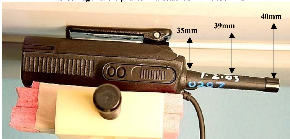
Figure 6: Assessment @ the Abdomen; DUT w/ belt clip HLN8255B against the phantom w/ attached HMN9030A RSM
