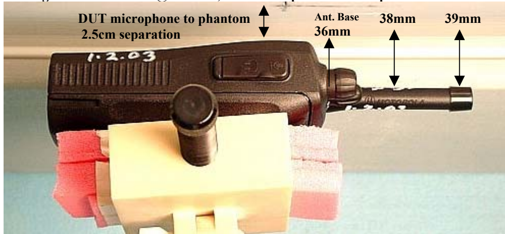
Figure 2. Assessment @ the face; DUT microphone 2.5cm separation distance
