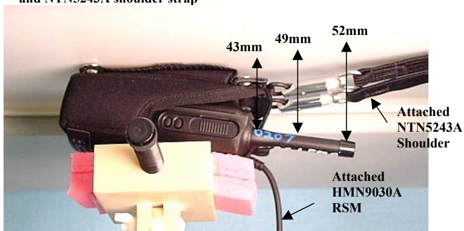
Figure 9: Assessment @ the Abdomen; DUT w/ carry accessory HLN9701B against the phantom w/ attached HMN9030A RSM, and NTN5243A shoulder strap
