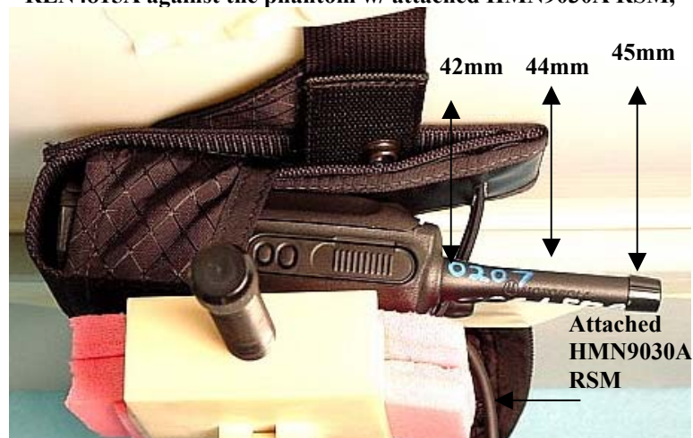
Figure 10: Assessment @ the Abdomen; DUT w/ carry accessory RLN4815A against the phantom w/ attached HMN9030A RSM,
