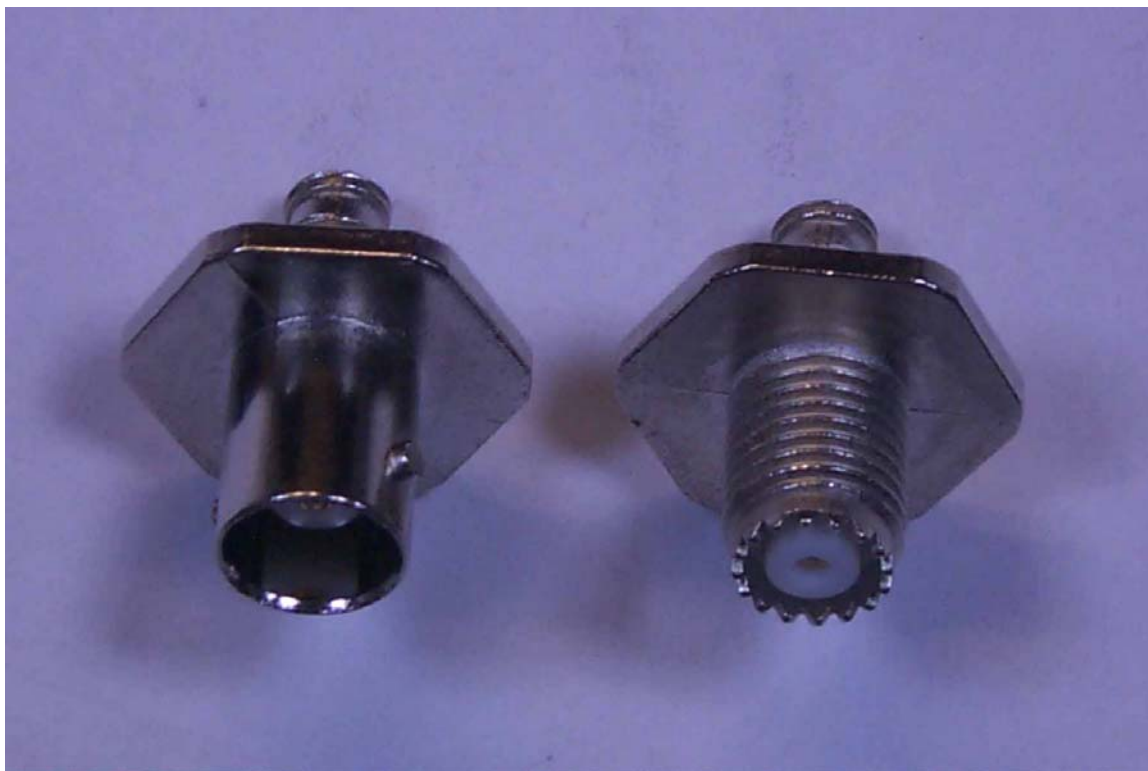
Figure 3-6: Antenna connector options, BNC on left, mini-UHF on right.
