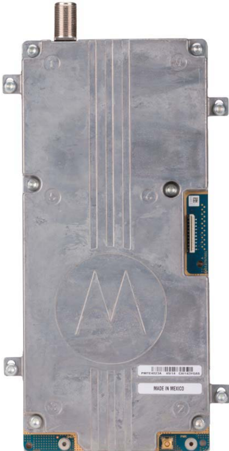
Internal Front View – Power Amplifier Module
