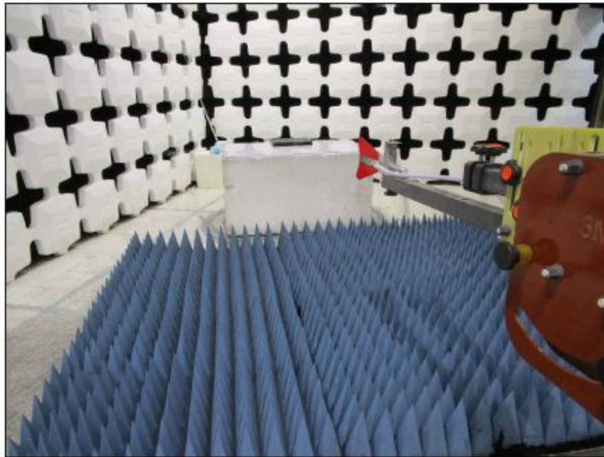
Test Setup for Radiated Emissions: 1GHz to 2GHz, Horizontal Polarization
