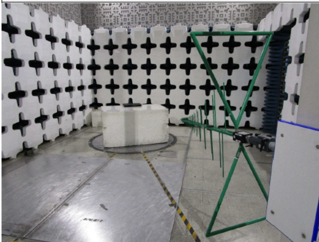
Test Setup for Radiated Emissions: 30MHz to 1GHz, Vertical Polarization
