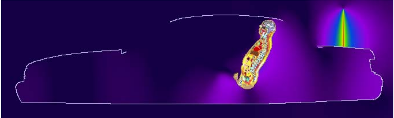
Figure 4. (a) E-field distribution corresponding to exposure condition of Figure 3, and (b) H-field distribution corresponding to exposure condition of Figure 3.
