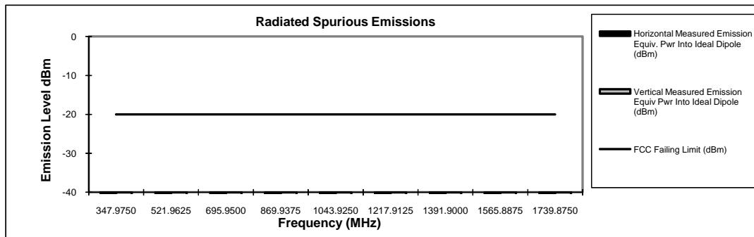
\* Indicates the spurious emission could not be detected due to noise limitations or ambient.
