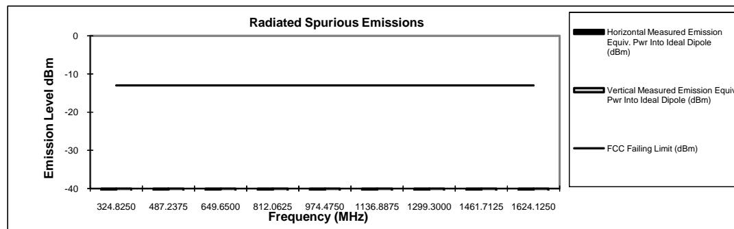
**Transmit Radiated Spurious Emissions: PMUD3241AABNAA**
