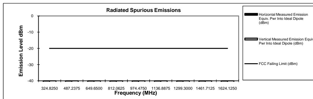
Transmit Radiated Spurious Emissions: PMUD3241AABNAA
