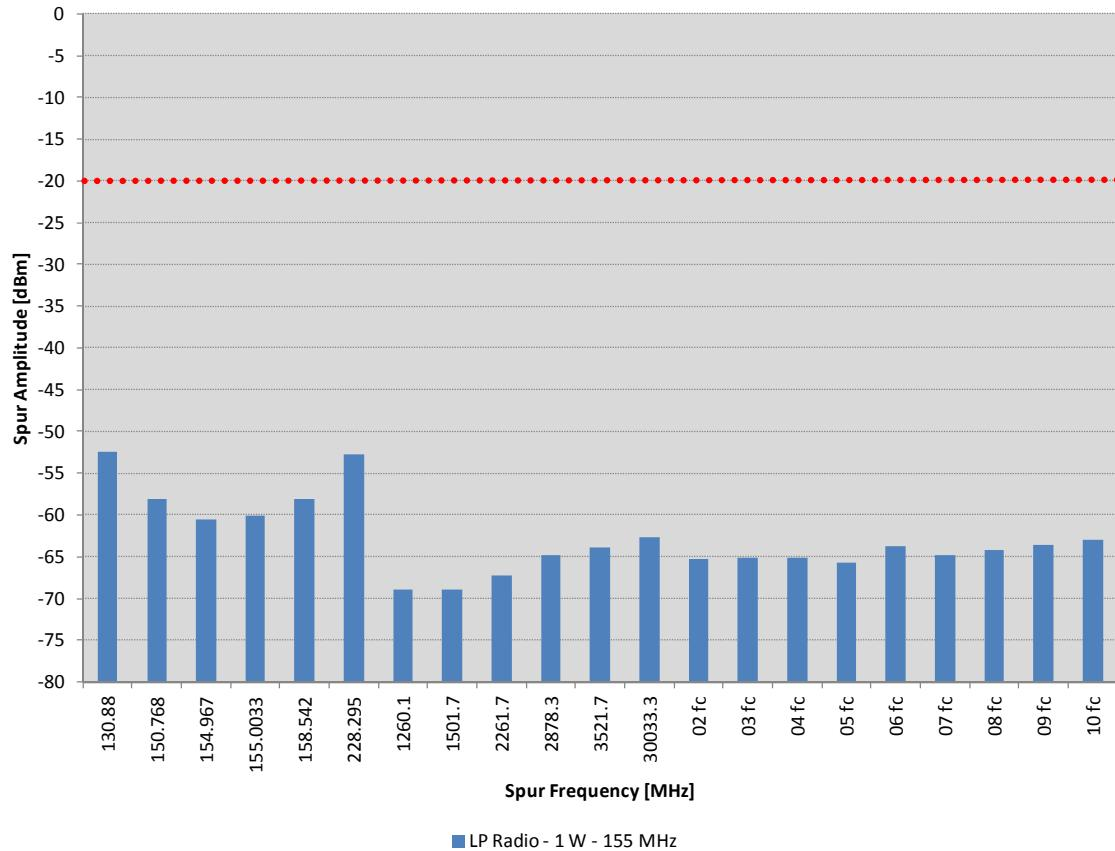
The conducted spurious level is plotted in dBm on the vertical axis.
