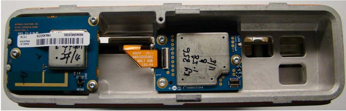
FRONT VIEW WITH BLUETOOTH/GPS BOARD INSTALLED ON THE LEFT AND GENERIC OPTION BOARD INSTALLED ON THE RIGHT
