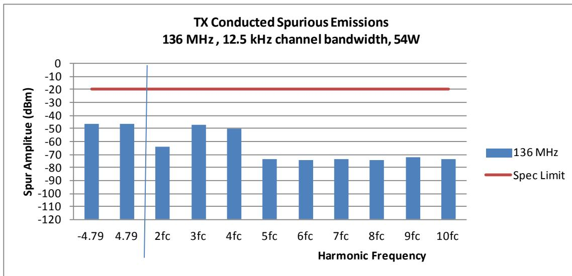
The conducted spurious level is plotted in dBm on the vertical axis.
