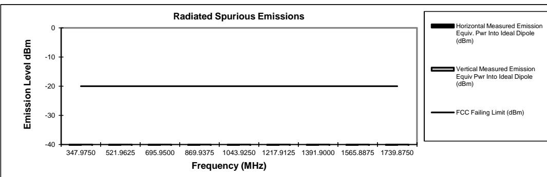
\* Indicates the spurious emission could not be detected due to noise limitations or ambient.
