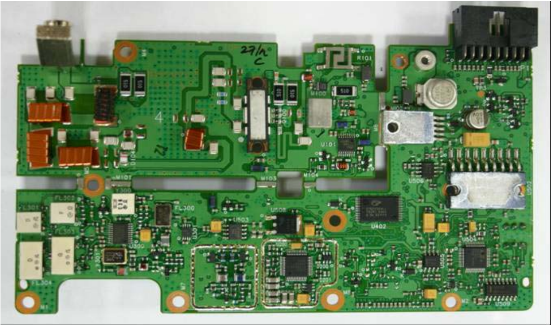
Figure 9-1: Top Side of PCB without shields.
