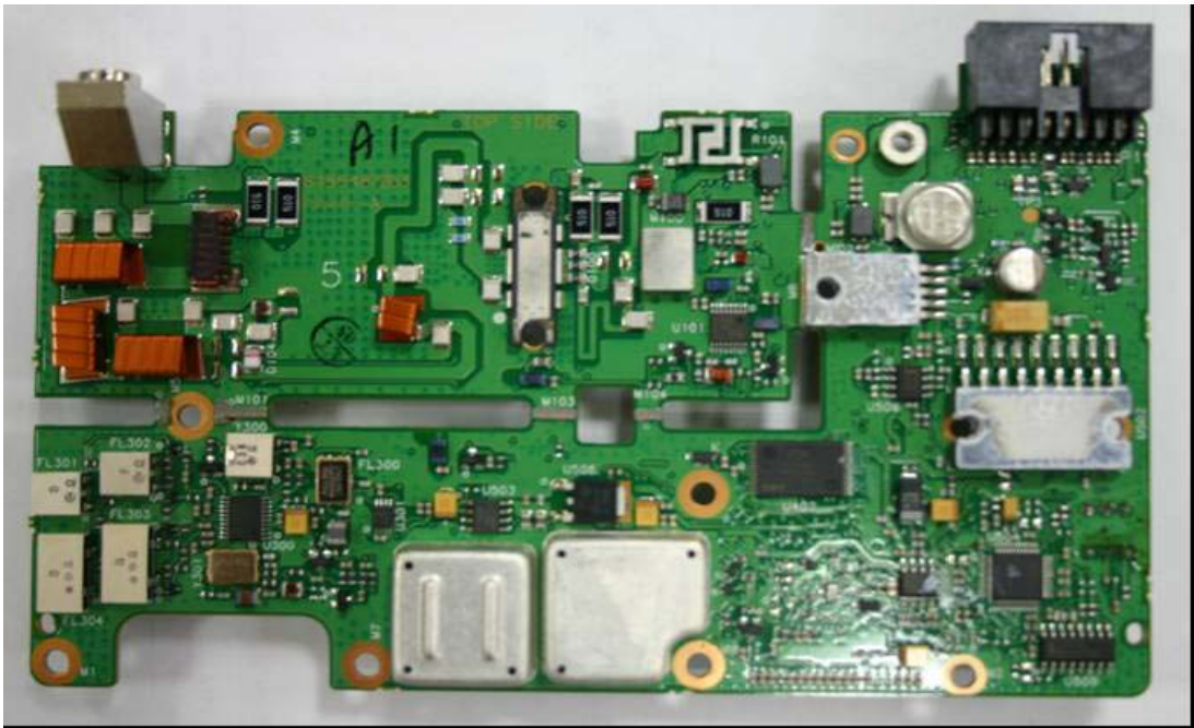
Figure 9-3: Top Side of PCB with shields.
