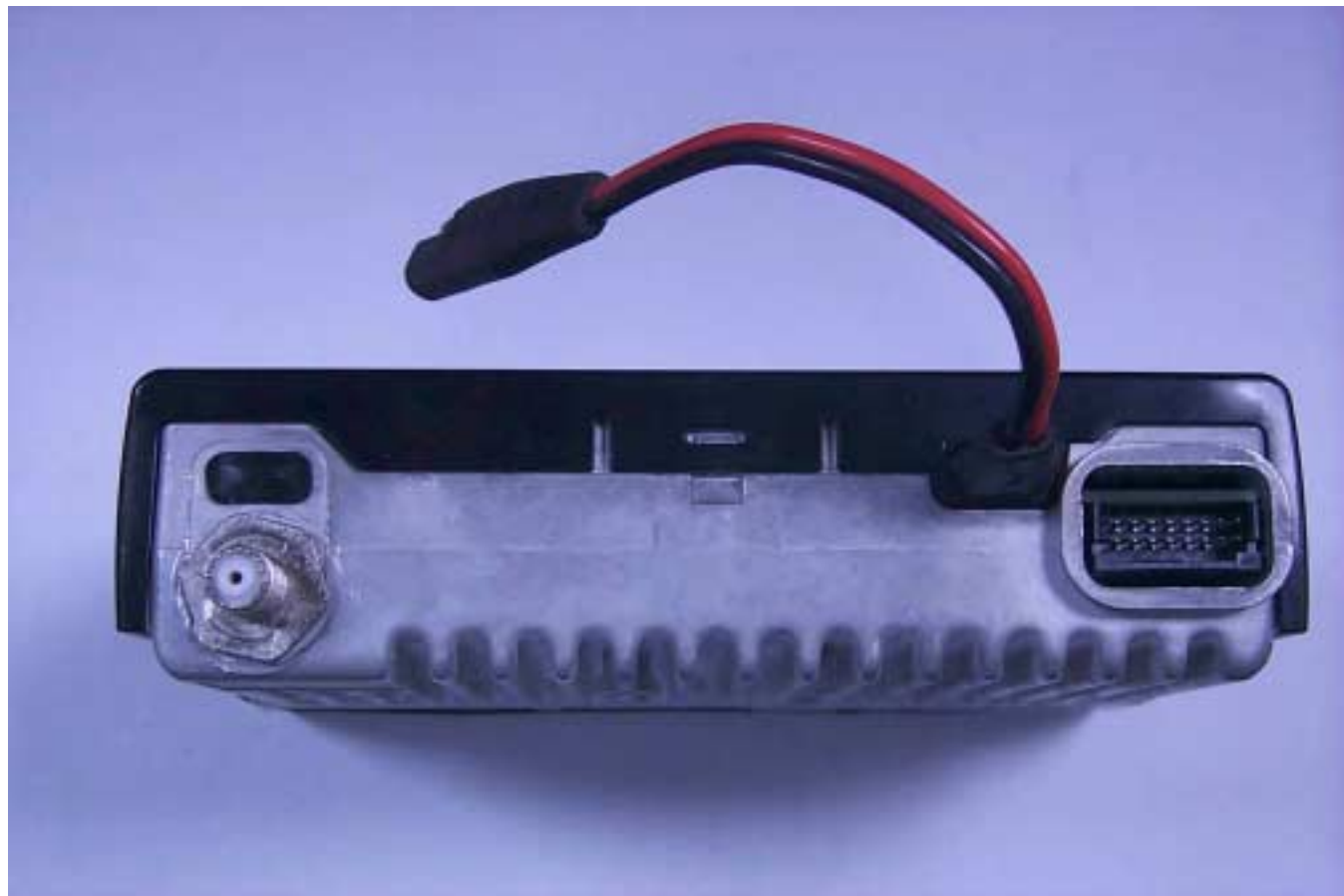
REAR VIEW SHOWING ANTENNA CONNECTOR, DC CABLE, AND ACCESSORY CONNECTOR
