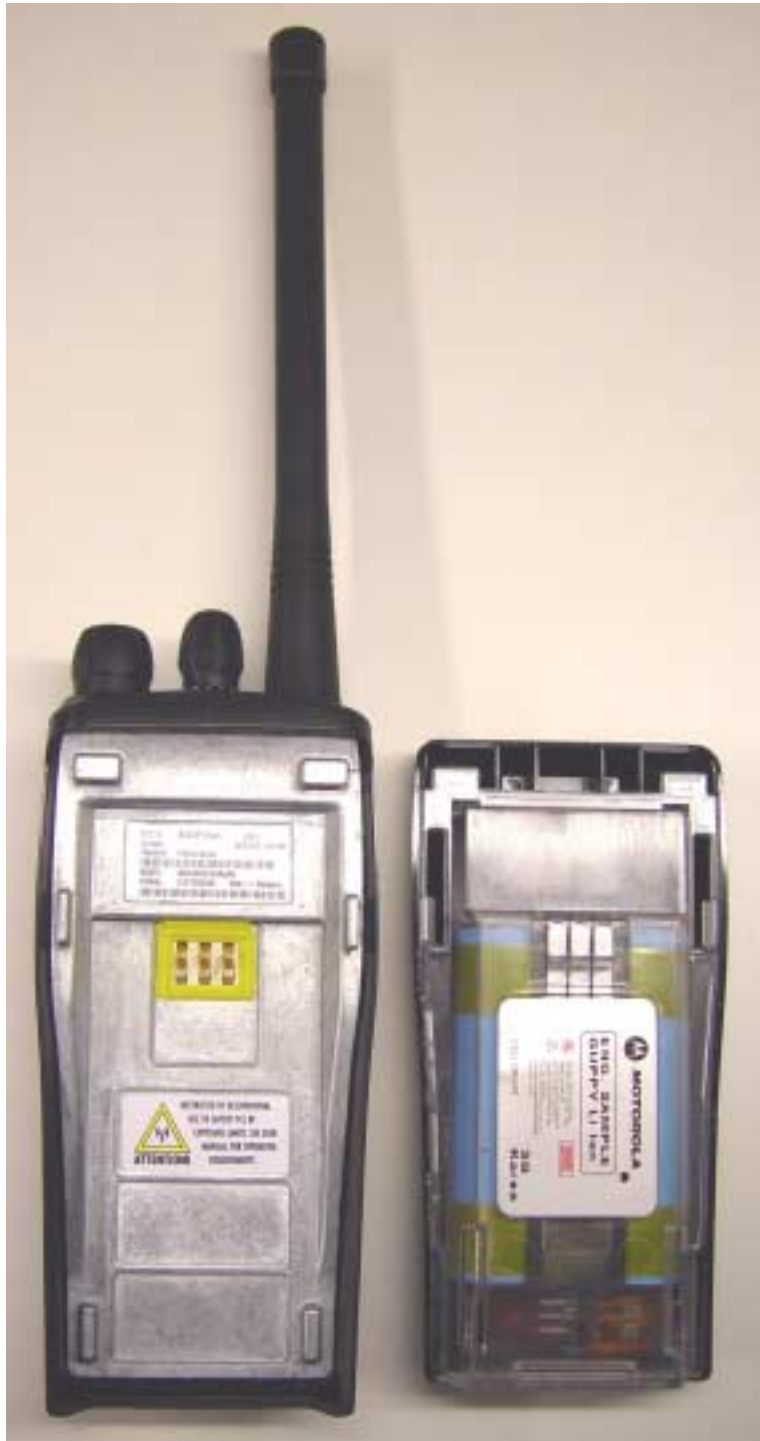
REAR VIEW WITH BATTERY REMOVED SHOWING FCC ID LABEL AND RF SAFETY LABEL
