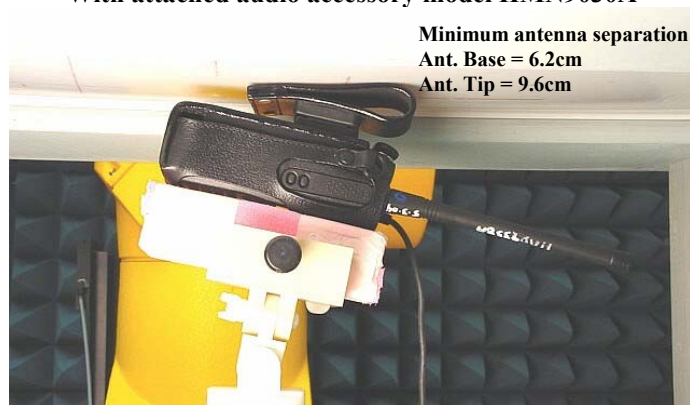
Figure 8. Assessment @ Body DUT with body worn accessory model RLN5497A against the phantom With attached audio accessory model HMN9030A
