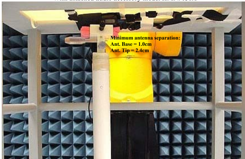
Figure 3. Assessment @ the body DUT with body worn accessory model HLN6602A against the phantom With attached audio accessory model HMN9030A
