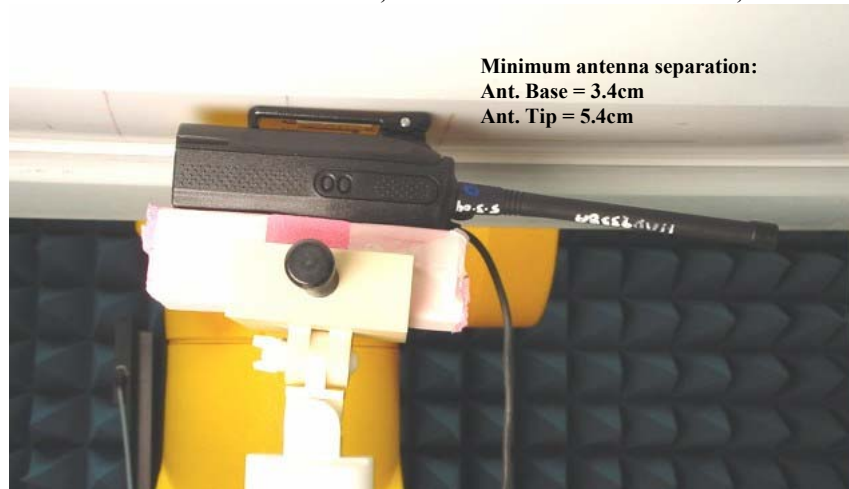
Figure 3. Assessment @ the body DUT with body worn accessory model HLN6602A against the phantom With attached audio accessory model HMN9030A
