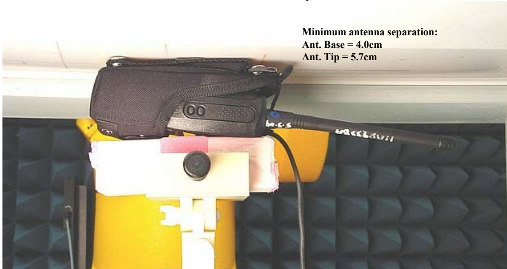
Figure 4. Assessment @ body DUT with body worn accessory model HLN9701B against the phantom With attached audio accessory model HMN9030A
