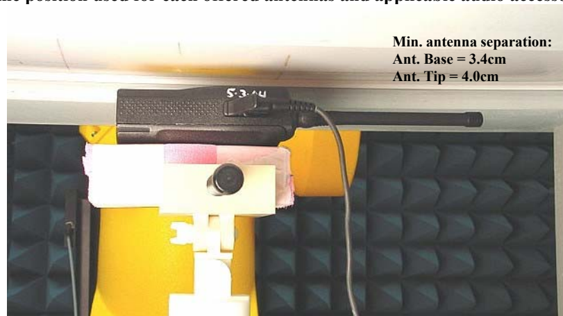
Figure 13: Robot Test System (Flat Phantom)
