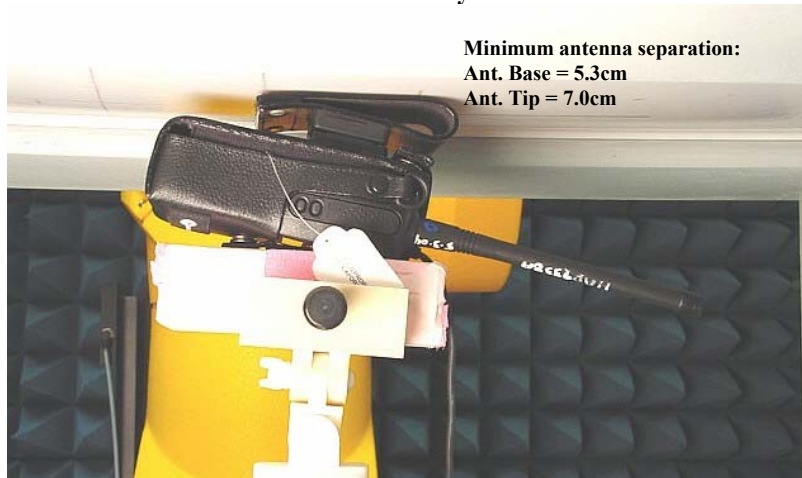
Figure 7. Assessment @ Body DUT with body worn accessory model RLN5644A against the phantom With attached audio accessory model HMN9030A
