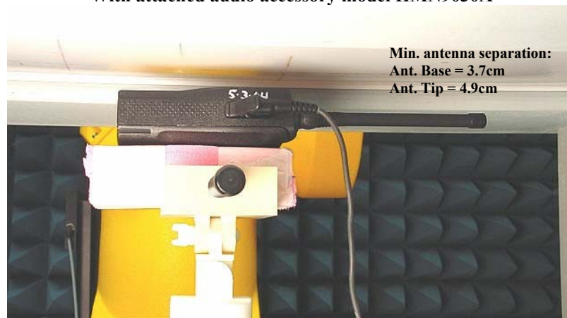
Figure 11. Assessment at the Body w/ front housing @ 2.5cm With attached audio accessory model HMN9030A
