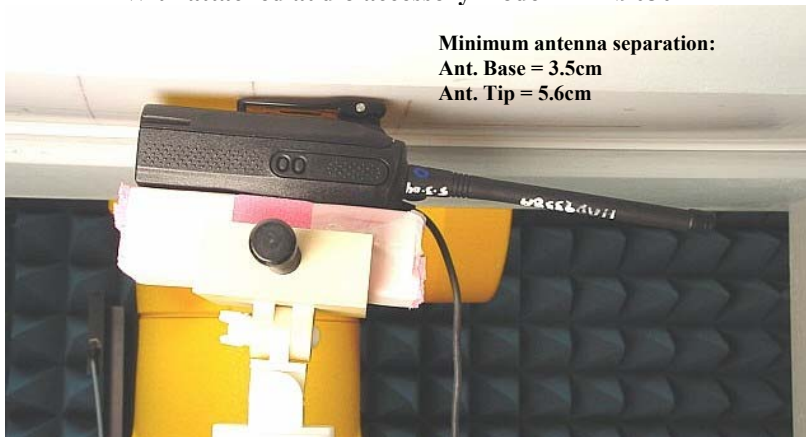
Figure 8. Assessment @ Body DUT with body worn accessory model RLN5497A against the phantom With attached audio accessory model HMN9030A
