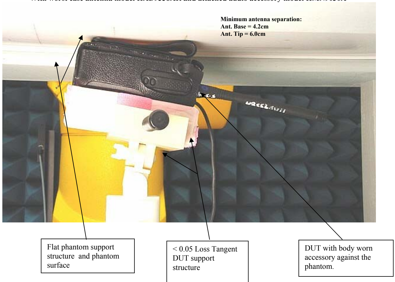
Figure 1: Highest S.A.R. Test Position (@ body) DUT with carry case model RLN5498A against the phantom With worst case antenna model HAD9338AR and attached audio accessory model HMN9030A
