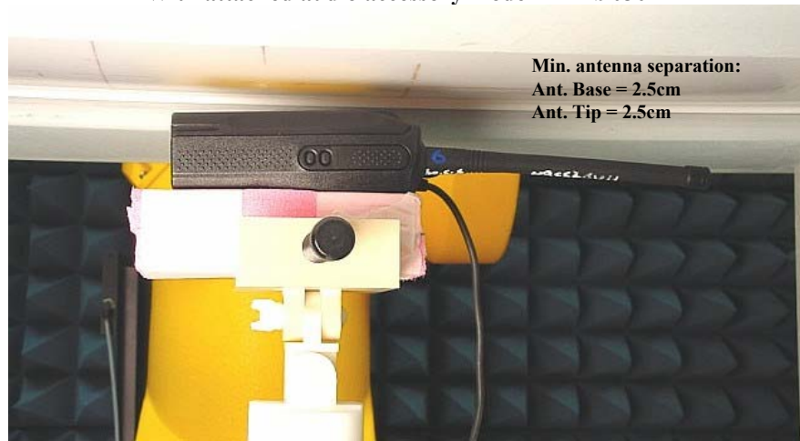
Figure 11. Assessment at the Body w/ front housing @ 2.5cm With attached audio accessory model HMN9030A
