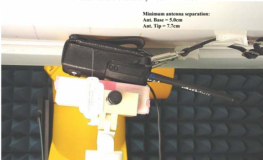
Figure 5. Assessment @ body DUT with body worn accessory model NTN5243A & RLN5383A against the phantom With attached audio accessory model HMN9030A
