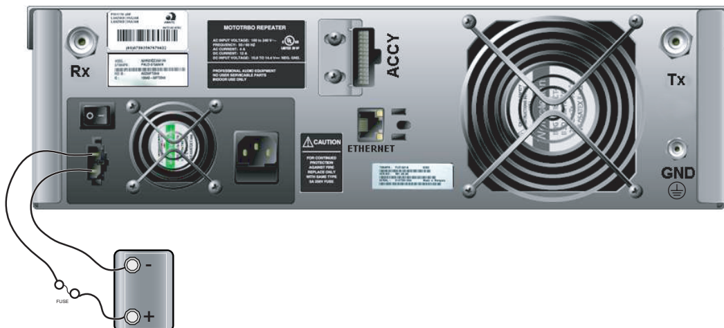
Figure 4-2 Making Connections to a Backup Battery
