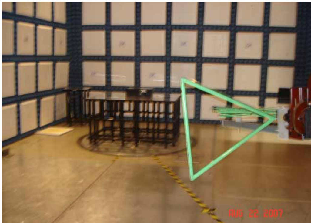
Test Set-up for Radiated Emissions, 30MHz to 1GHz - Horizontal Polarization
