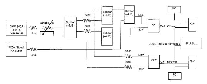
The SMU 200A generates a CW signal with a frequency within the AP operating frequency to create interference. The MXA Signal Analyzer monitors the AP output signal to visually show that AP stops transmission when interference is detected and resumes when interference goes away.
