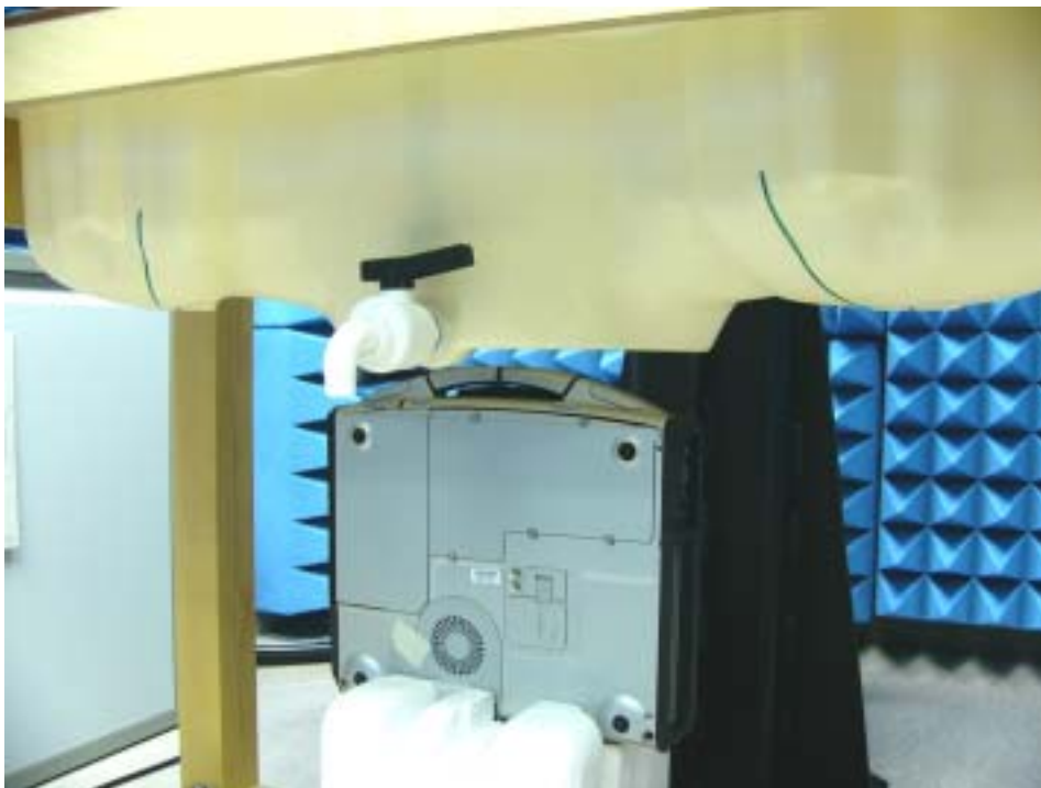
Fig.2 Photograph of the edge of the PC at 90° and at a distance of 1.5 cm from the base of the phantom
