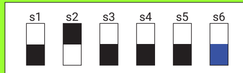
Figure 83: RMC Dip Switch Example - 29 dB in Normal Mode
