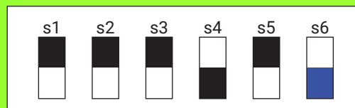
Figure 62: RMC DIP Switch Example - 8 dB Normal Mode
