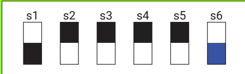
Figure 56: RMC DIP Switch Example - 2 dB Normal Mode
