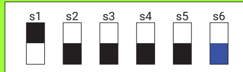
Figure 85: RMC Dip Switch Example - 31 dB in Normal Mode
