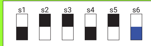
Figure 64: RMC Dip Switch Example - 10 dB in Normal Mode
