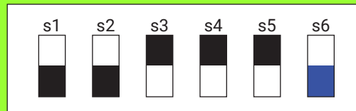
Figure 58: RMC DIP Switch Example - 4 dB Normal Mode
