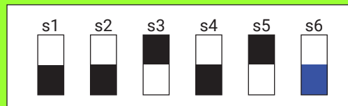
Figure 65: RMC Dip Switch Example - 11 dB in Normal Mode
