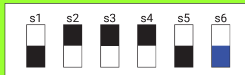
Figure 72: RMC Dip Switch Example - 18 dB in Normal Mode
