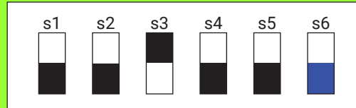
Figure 82: RMC Dip Switch Example - 28 dB in Normal Mode
