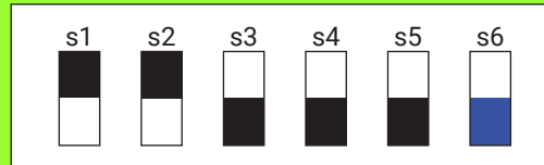
Figure 83: RMC Dip Switch Example - 29 dB in Normal Mode
