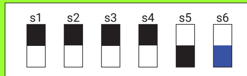
Figure 71: RMC Dip Switch Example - 17 dB in Normal Mode
