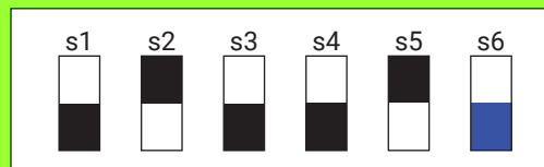
Figure 68: RMC Dip Switch Example - 14 dB in Normal Mode
