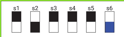
Figure 56: RMC DIP Switch Example - 2 dB Normal Mode
