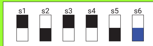
Figure 73: RMC Dip Switch Example - 19 dB in Normal Mode
