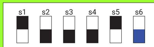
Figure 68: RMC Dip Switch Example - 14 dB in Normal Mode
