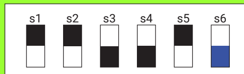
Figure 66: RMC Dip Switch Example - 12 dB in Normal Mode
