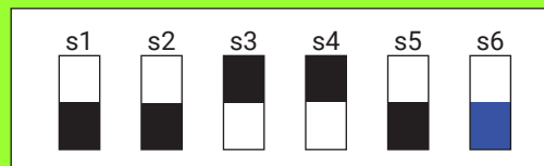
Figure 74: RMC Dip Switch Example - 20 dB in Normal Mode
