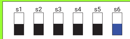
Figure 85: RMC Dip Switch Example - 31 dB in Normal Mode
