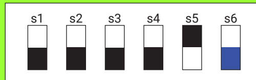
Figure 70: RMC Dip Switch Example - 16 dB in Normal Mode
