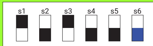
Figure 80: RMC Dip Switch Example - 26 dB in Normal Mode
