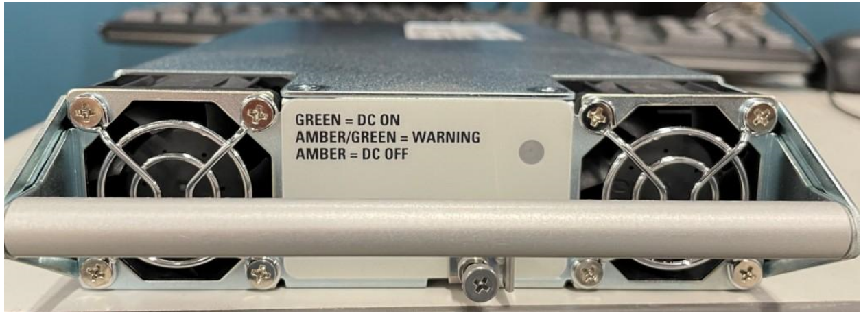
D2-4 Internal Front View - Power Amplifier Power Supply Module
