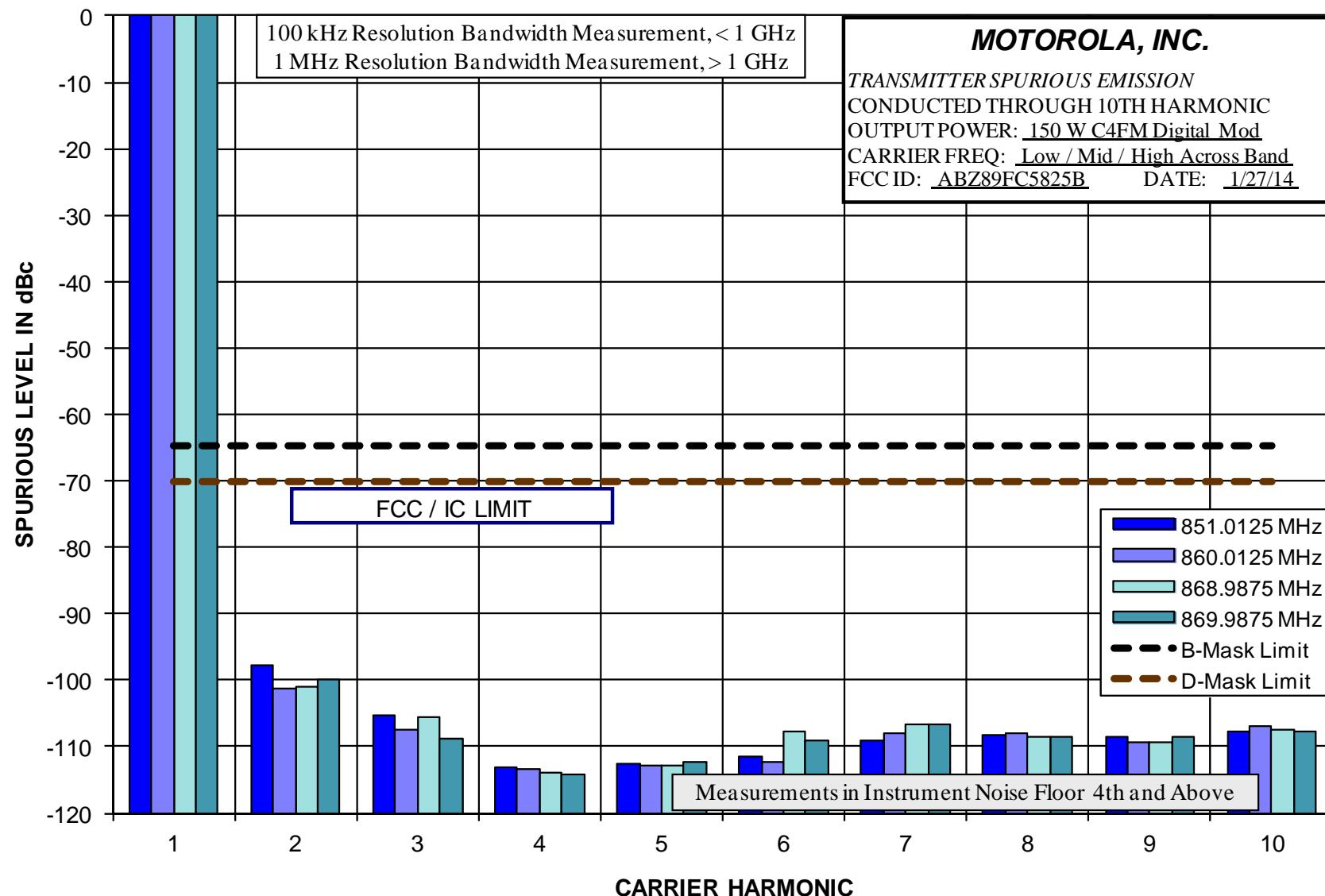
Conducted Spurious Harmonic Emissions – 15 Watts C4FM
