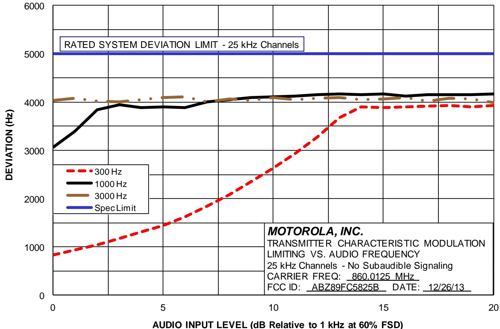
Modulation Limiting – 25 kHz Channels – High End of Band
