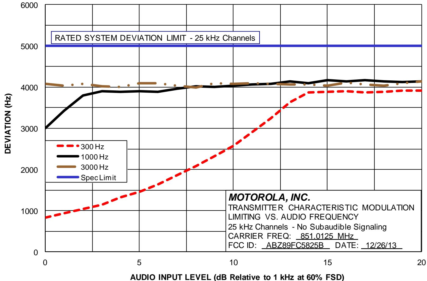
Modulation Limiting – 25 kHz Channels – Middle of Band
