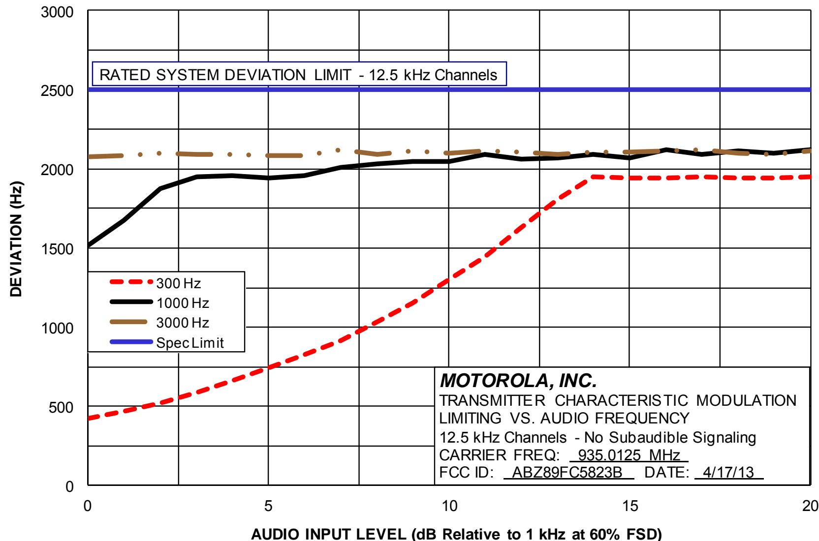
Modulation Limiting – 12.5 kHz Channels – Middle of Band
