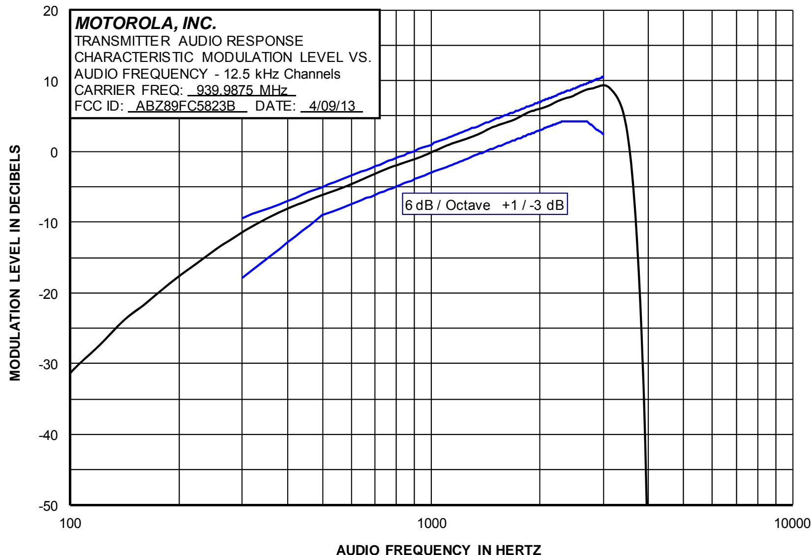
**Report on Test Measurements***Modulation Limiting*Specification Requirement per TIA 603:
