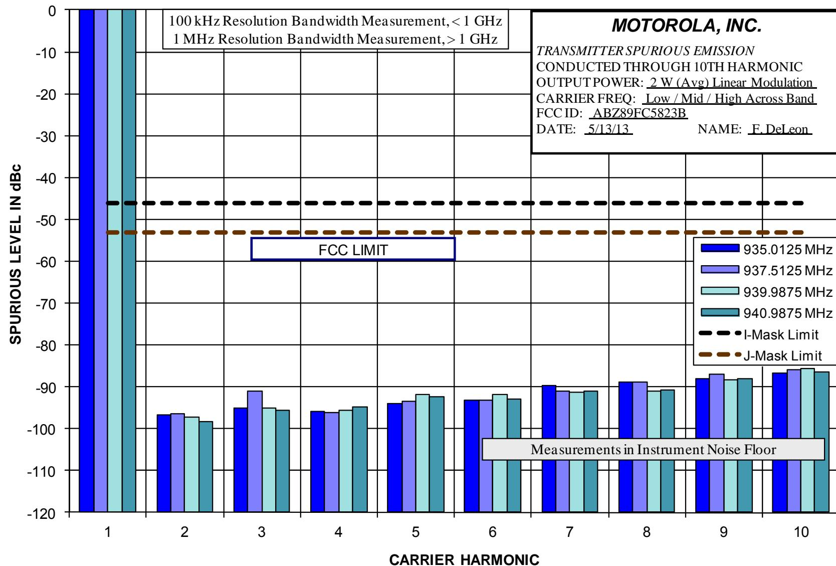
Conducted Spurious Harmonic Emissions – 120 Watts C4FM
