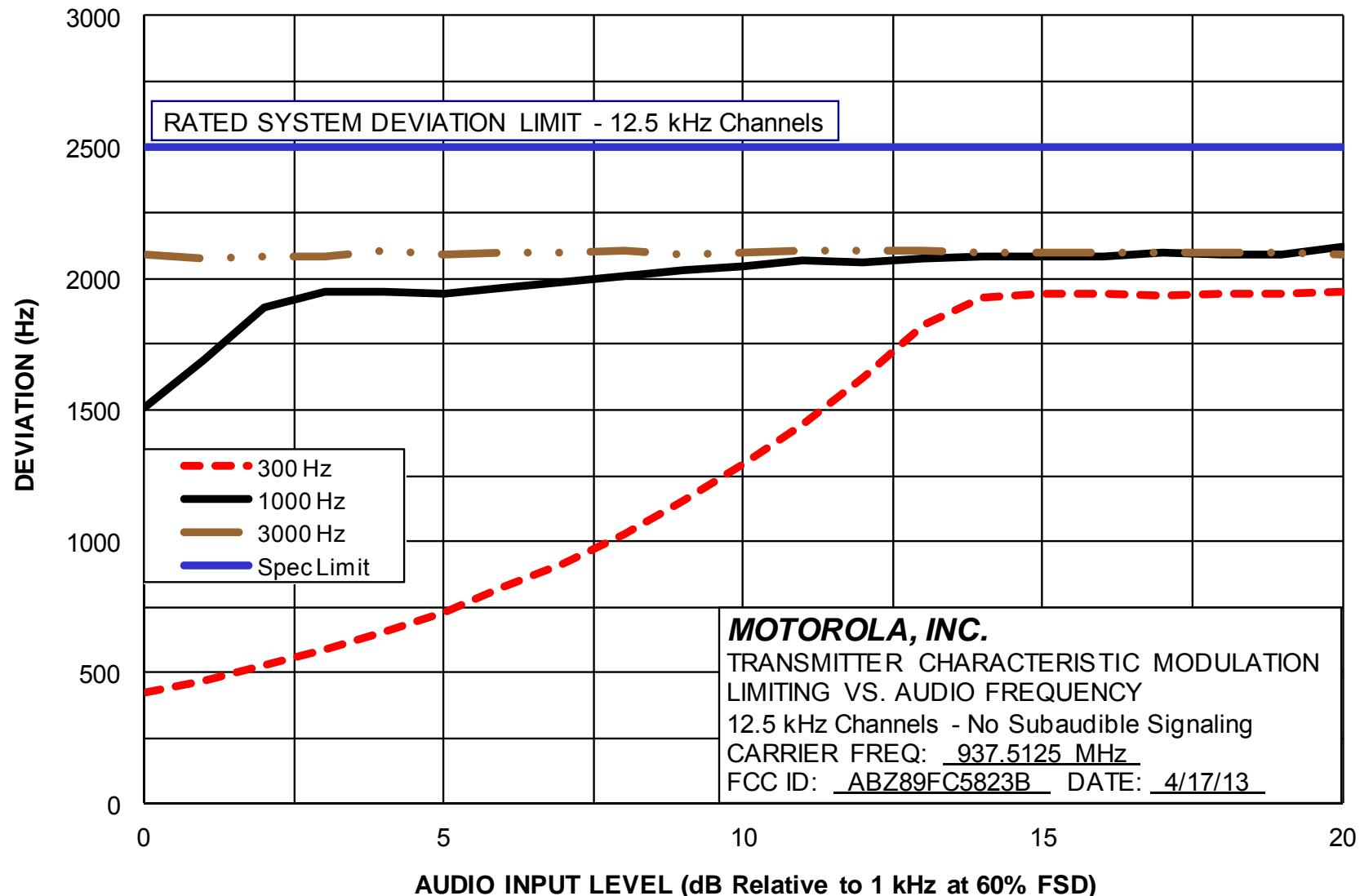
Modulation Limiting – 12.5 kHz Channels – High End of Band
