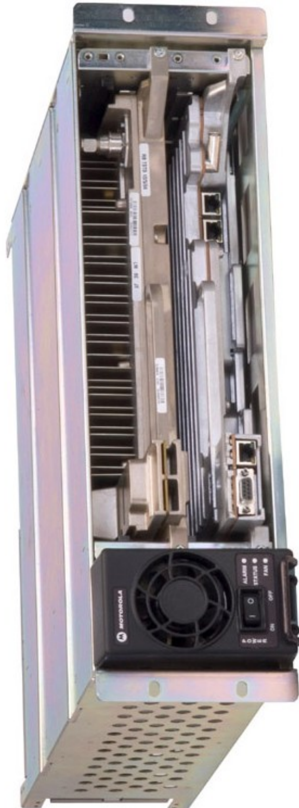
External Front View of Base Radio, Front Panel Removed
