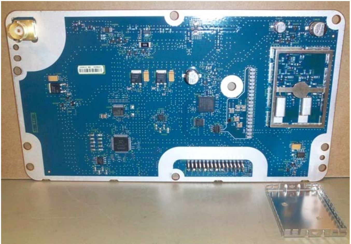
Internal Front View – Exciter Board, Top View
