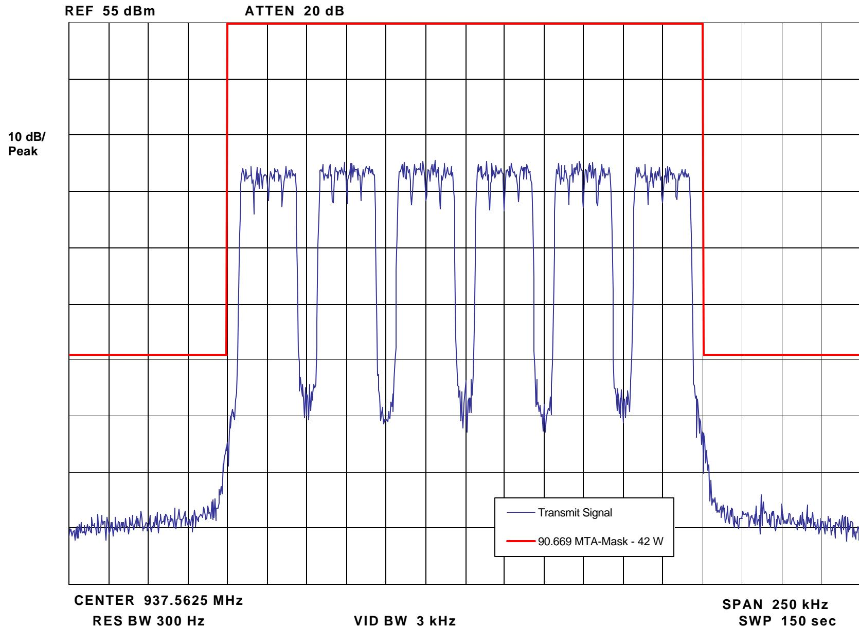
**Report on Test Measurements***Conducted Spurious Emissions, Harmonics and Close-In, 800 MHz Operation***§ 90.691 Emission Mask Requirements for EA-Based Systems:**
