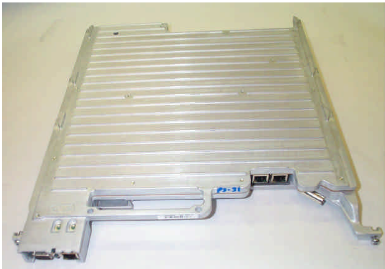
Internal Front View – Transceiver Module
