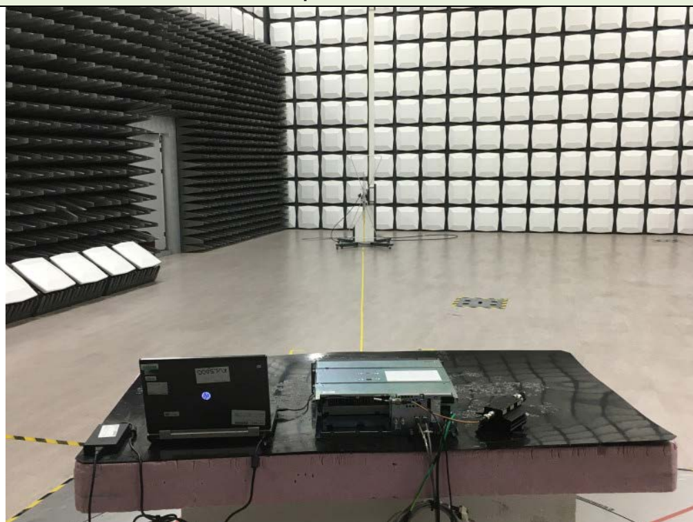
Test Setup for 30 MHz – 1 GHz
