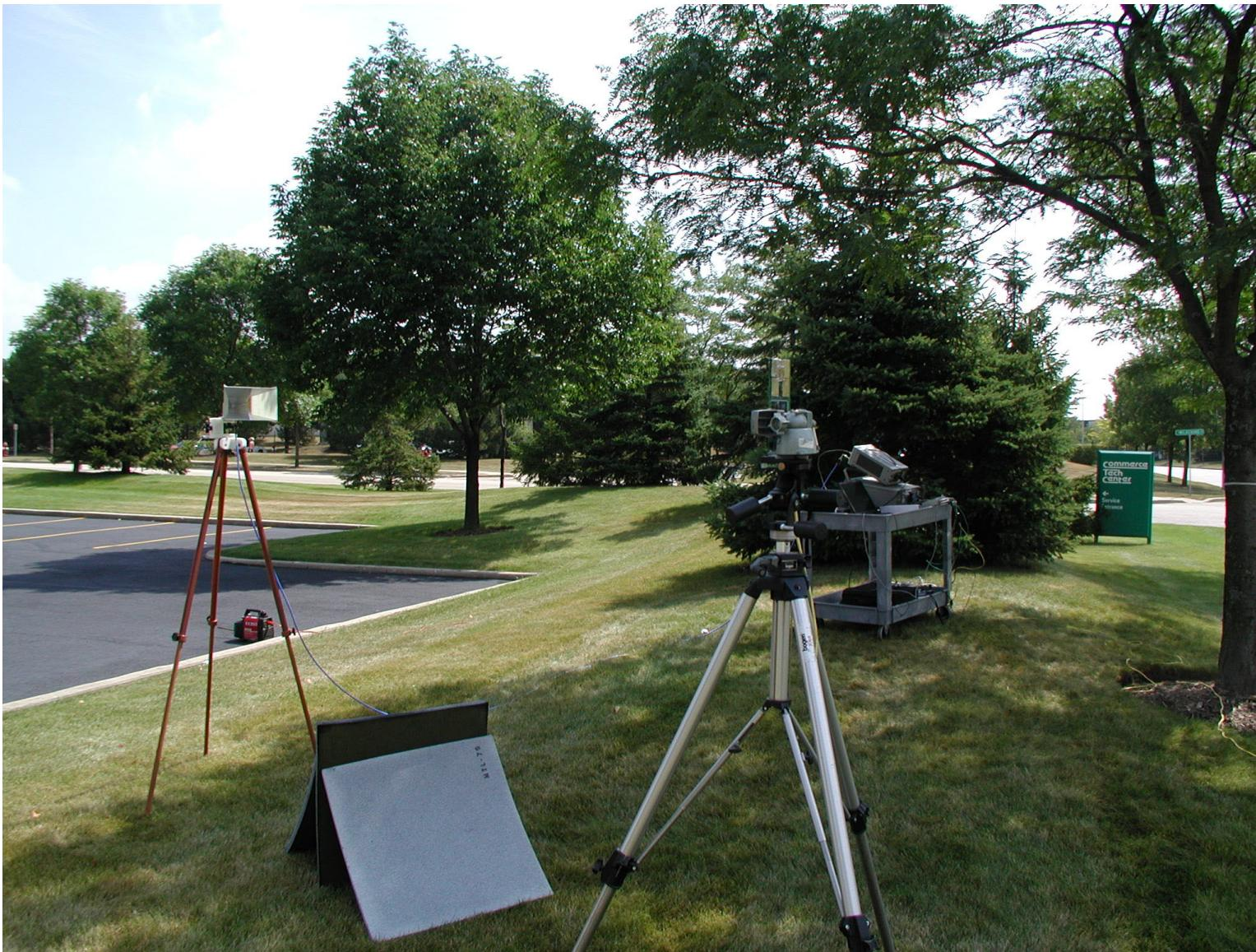
The test antenna and test radio were mounted on adjustable tripods and placed 3 meters apart. Absorbing panels were placed on the ground to reduce the effects of ground reflections.
