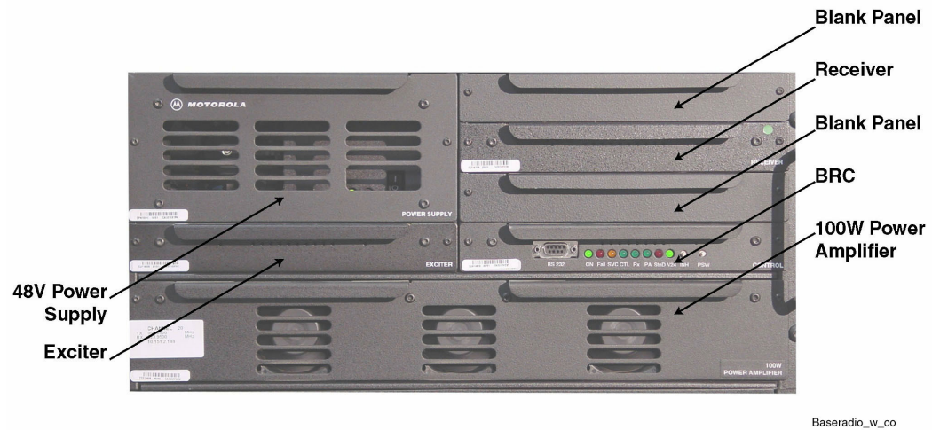
Figure 5-3 Layout of the Base Radio Modules
