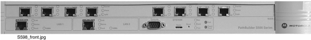
Figure 5-20 Front View of the Simulcast Remote Site Router
