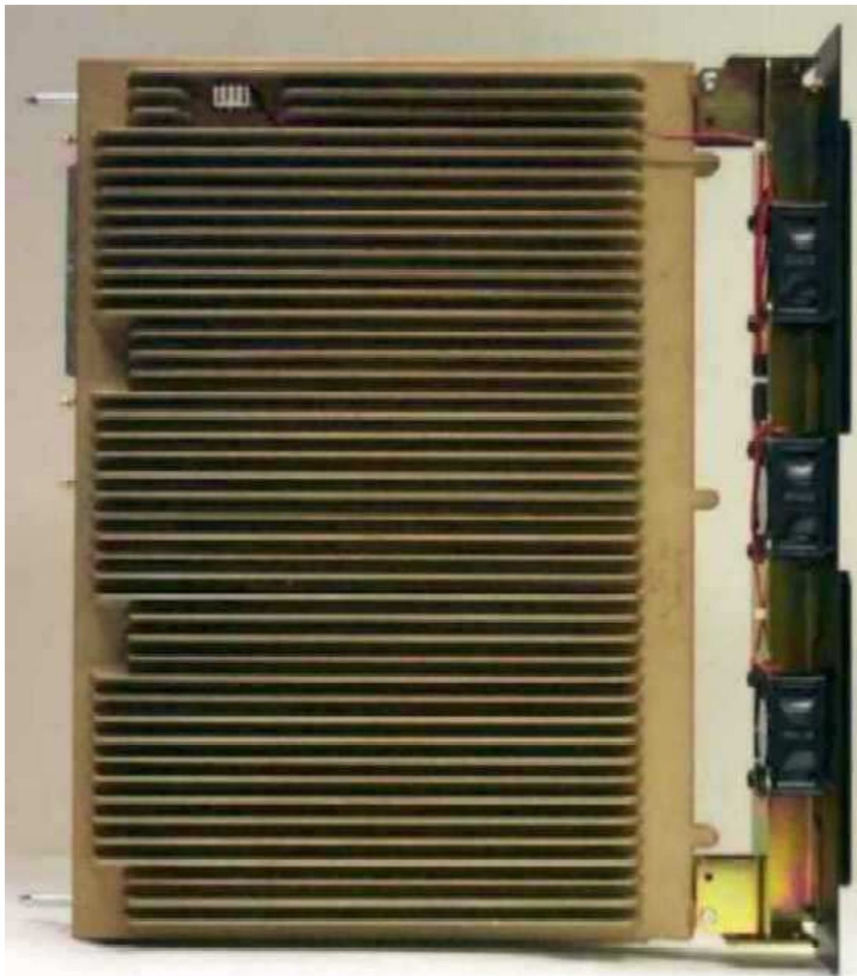
Power Amplifier Module, Heat Sink View
