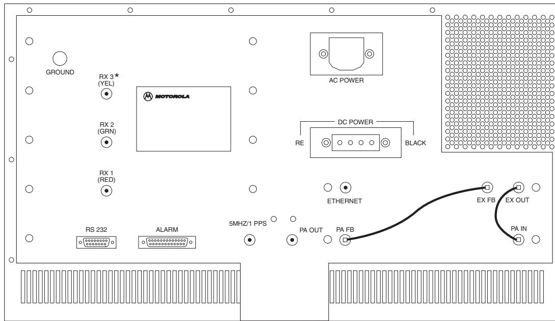
\* This port must be terminated by  $50\Omega$  load when configured for 2 Branch Diversity. Also, the rx\_fru\_config parameter must be set to R12.
