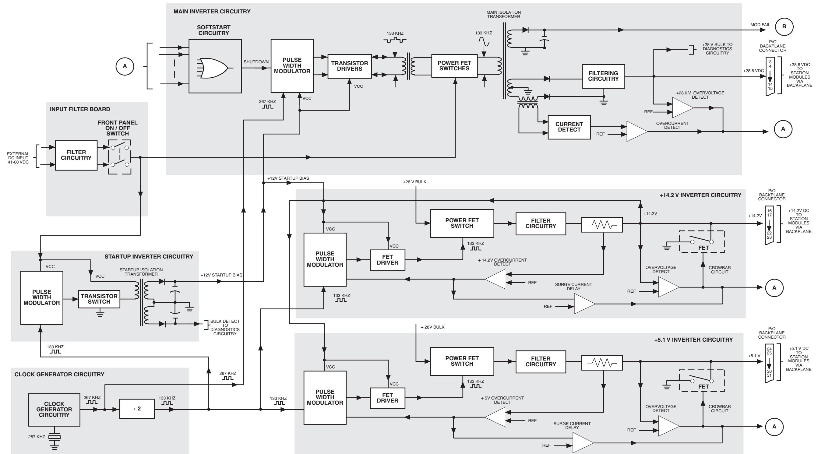
Figure 5 QUAD BR DC Power Supply (Sheet 1 of 2)
