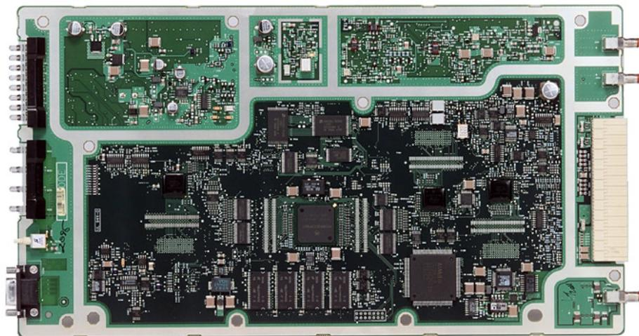
Figure 4 900 MHz QUAD Channel Exciter (with cover removed)
