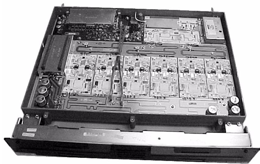
Figure 5    **800/900 MHz QUAD PA**
