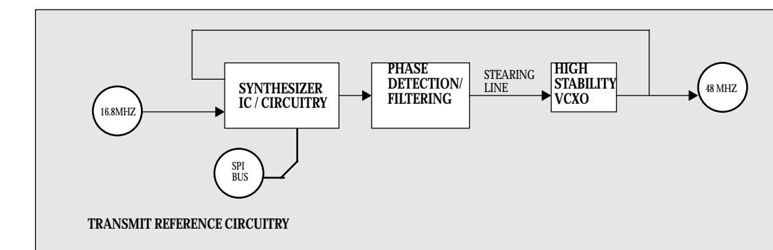
Figure 13 800 and 900 MHz QUAD Channel Base Radio Controller Functional Block Diagram (Sheet 1 of 2)
