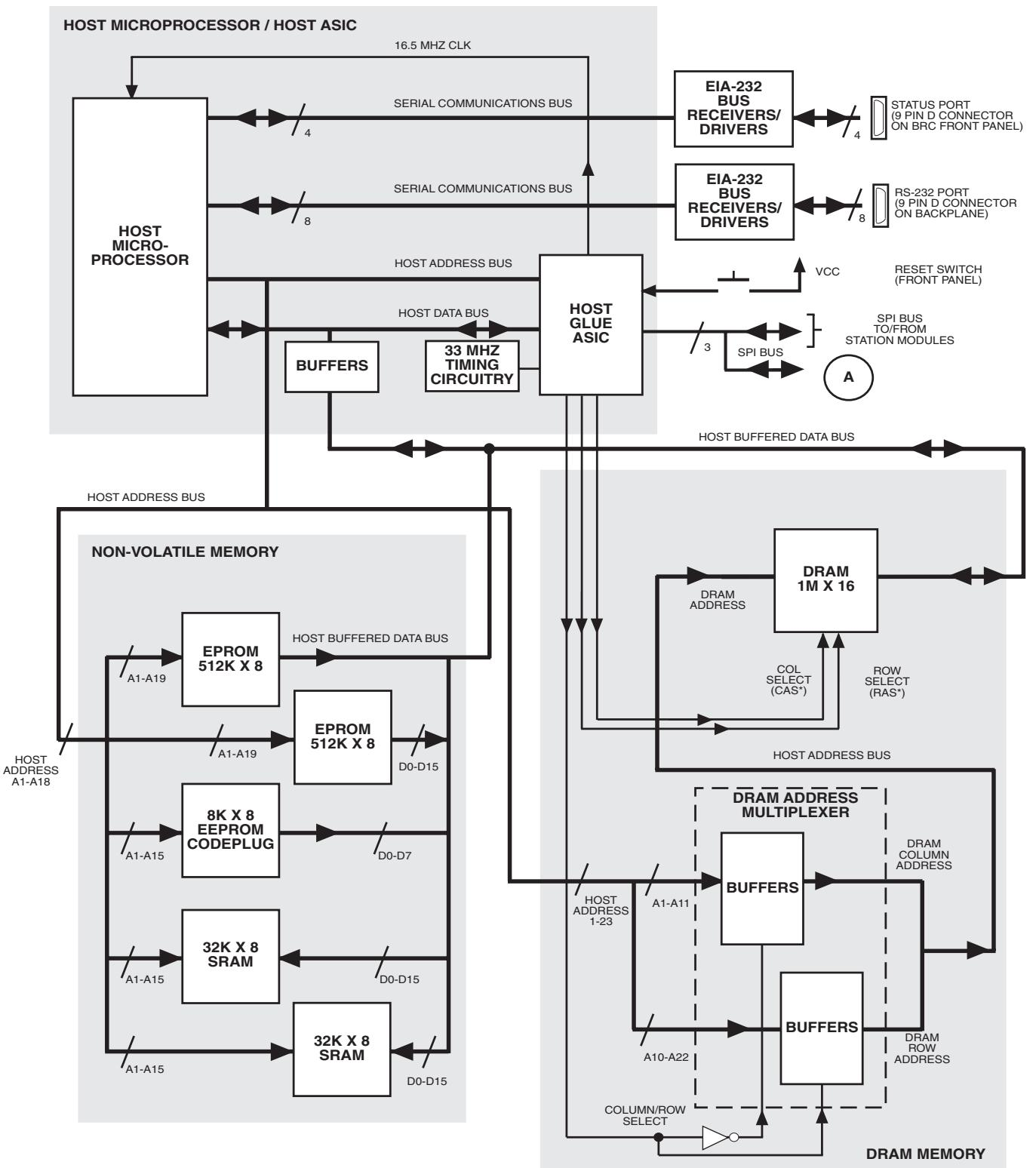
Figure 10 800/900 MHz Base Radio Controller Functional Block Diagram
