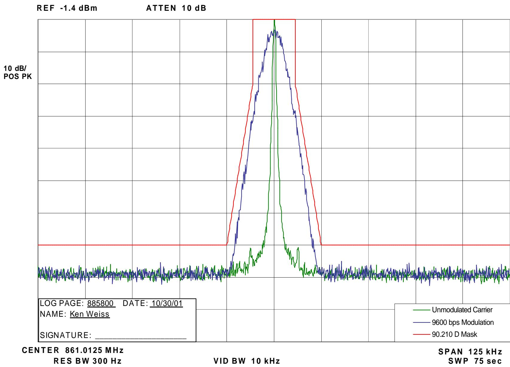
Occupied Bandwidth - 12.5 kHz Channels - Carrier with 9600 bps Digitized Voice -
