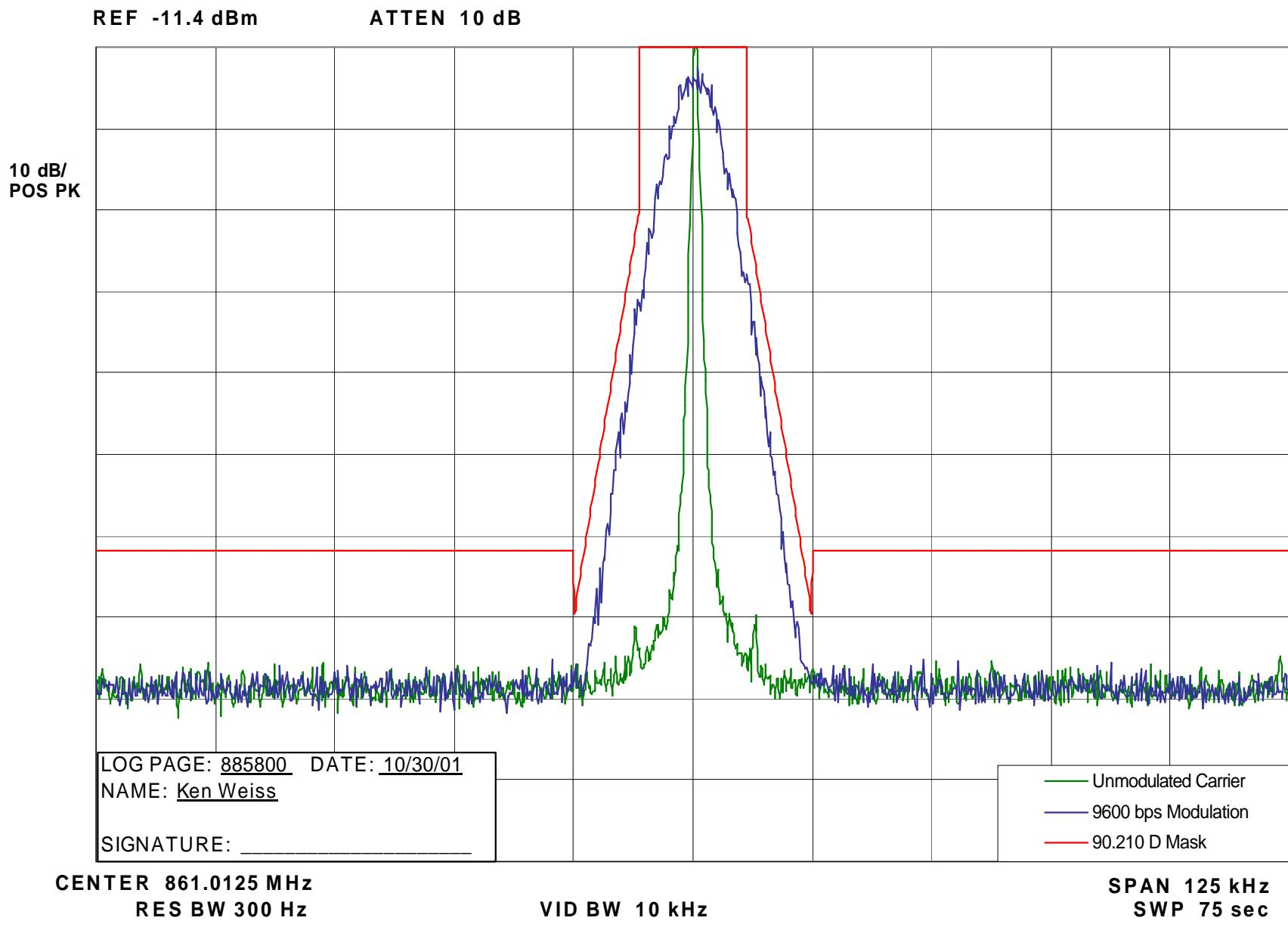
**CONDUCTED SPURIOUS EMISSIONS****SPECIFICATION REQUIREMENT:****Reference: Part 90.210 (Emission Mask B, C)**
