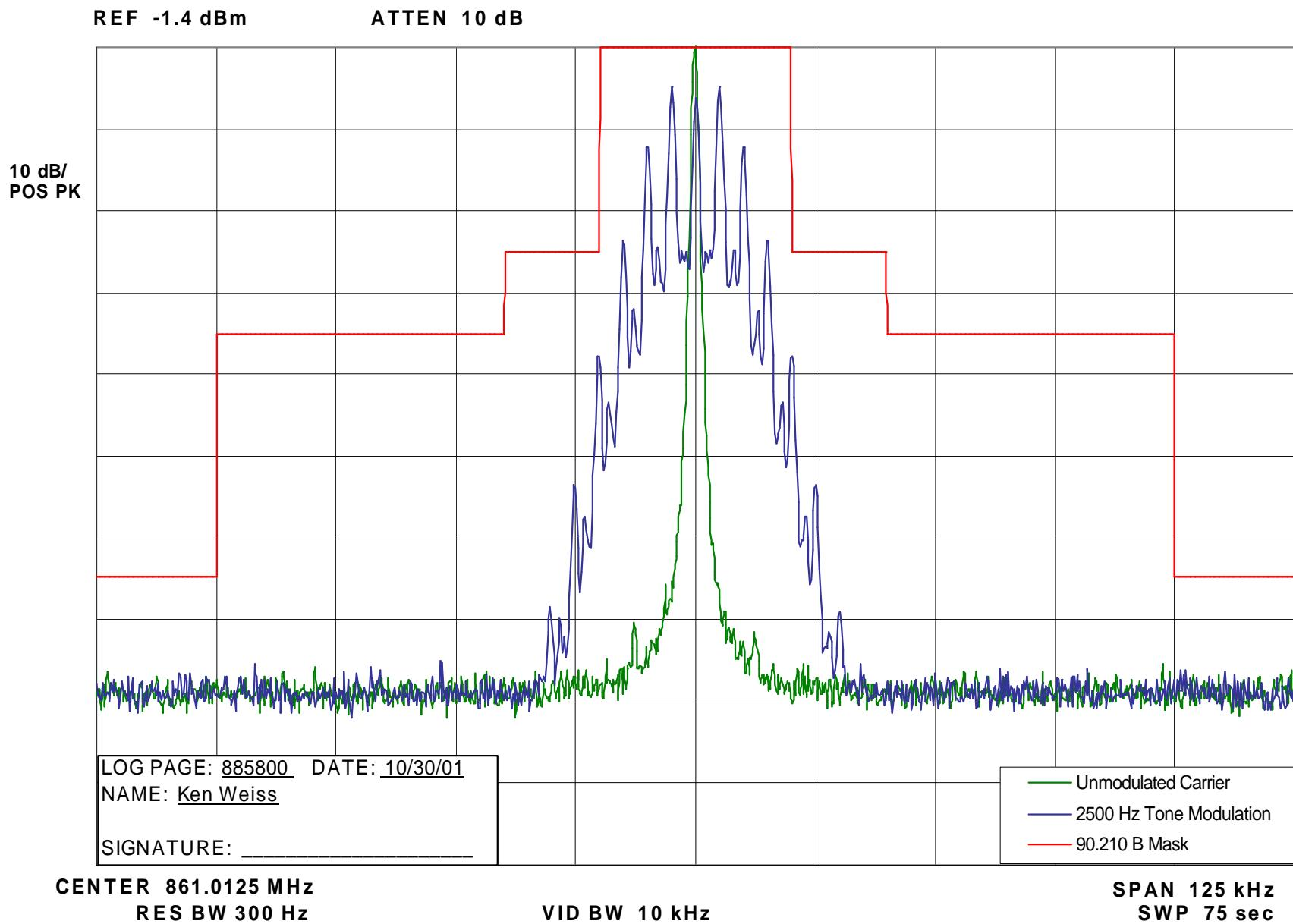
Occupied Bandwidth - 25 kHz Channels - Carrier with 2500 Hz Audio Tone -
