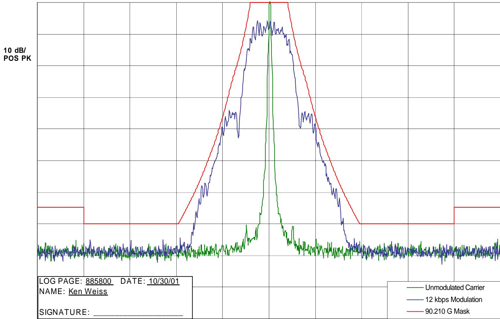
Occupied Bandwidth - 25 kHz Channels - Carrier with 12 kbps Digitized Voice -
